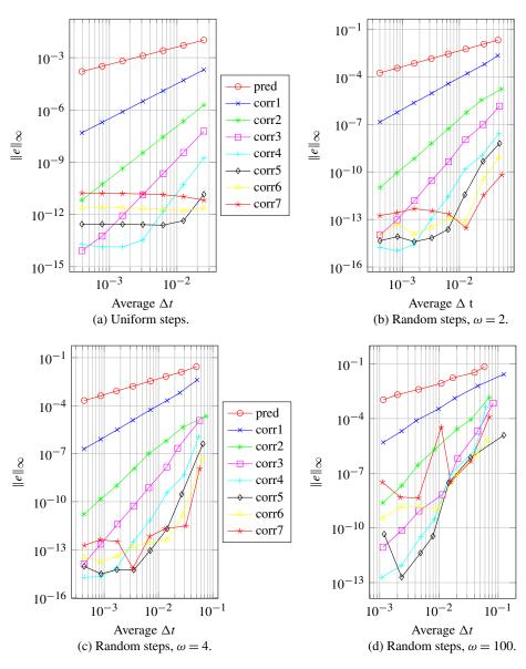
Figure 3. Auzinger IVP: The design order is illustrated for the RIDC methods.
