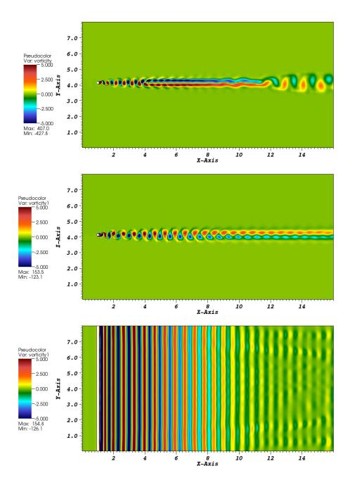
**Figure 14.** Flow past a cylinder at Re = 300. Top: 2D simulation of vorticity. Middle: 3D simulation of *y* vorticity in the *x*-*z* plane at z = 4.125. Bottom: 3D simulation of *y* vorticity in the *x*-*y* plane at y = 4. The cylinder has radius r = 0.0625 and is shown in white centered at x = 1, y = 4.125 in 2D and x = 1, y = 4, z = 4.125 in 3D. Time simulated is 98 seconds.
