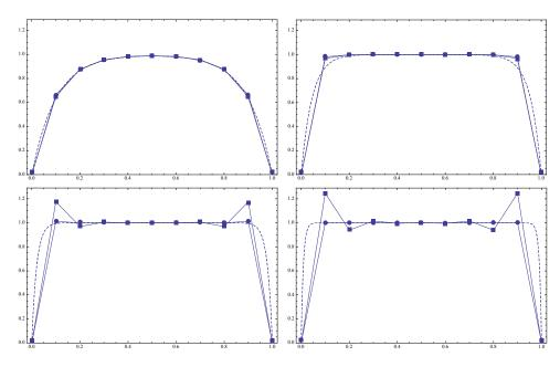
**Figure 3.** Standard Galerkin (squares) and weighted Galerkin (circles) approximations to (3-2) for c = 100, 500, 2500, 12500 with exact solutions (dashed).
