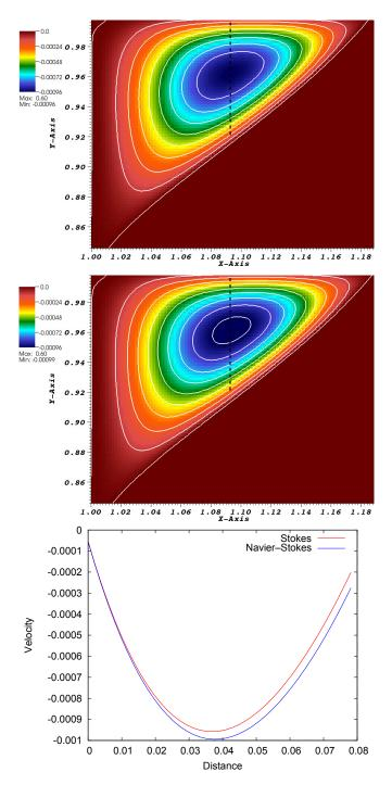
**Figure 6.** Zoomed-in view of the recirculation zone in the corner behind the backwardfacing step for Re = 0.1. Top: solution to the Stokes equation. Middle: solution to the Navier–Stokes equation. Bottom: plots of velocity along the dotted lines in the top figures.
