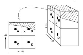
**Figure 2.** 3D bilinear flux interpolation stencil showing the interpolation point marked by an " $\times$ " for a 3D face in the  $\hat{e}^1$  direction using face-centered points A, B, C and D.
