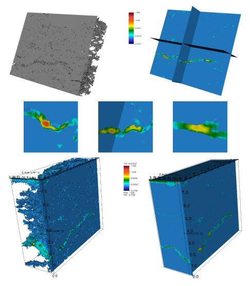
**Figure 13.** Steady-state flow through fractured shale: embedded boundary grid in gray (top left) with slices at mid-planes of *z*-velocity (top right), magnifications (middle) and rotated view of boundary data (bottom left) with slice planes near maximum velocity location (bottom right). Resolution is h = 48.4 nm with  $1920 \times 1600 \times 640$  total grid cells and 18% porosity. Inlet velocity is 0.008 cm/sec. Computation was performed on NERSC Hopper using 60,000 processor cores.
