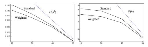
Figure 5.  $L^2$  norm and  $H^1$  seminorm errors for 2D convection-dominated diffusion problem.
