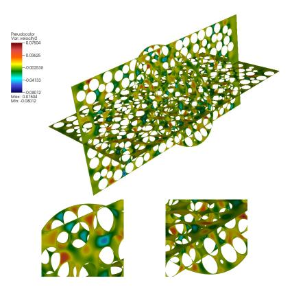
**Figure 10.** Steady-state flow through the packed cylinder geometry in Figure 7 (middle). Transverse (*z*) velocity shown with magnified views of the top and bottom of the cross-sectional slice. Inlet axial velocity is 0.01 cm/sec with Re = 0.5. Computation was performed on NERSC Cray XC30 Edison using 65,536 processor cores.
