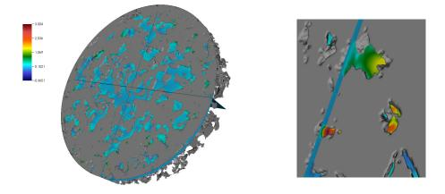
**Figure 12.** Steady-state flow through Bedford limestone: embedded boundary grid in gray with *z*-velocity data (left) and magnification of the bottom of the disk (right). Resolution is h = 43 nm with 2048 × 2048 × 320 total grid cells and 29% porosity. Inlet velocity is 0.0376 cm/sec. Computation was performed on OLCF Titan using 40,960 processor cores.
