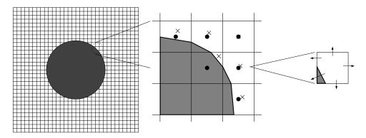
**Figure 1.** Left: example of an irregular geometry on a Cartesian grid. Middle: close-up view of embedded boundaries "cutting" regular cells. Right: single cut cell showing boundary fluxes. The shaded area represents the volume of cells excluded from the domain. Dots represent cell centers. Each "×" represents a centroid.
