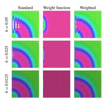
**Figure 4.** Numerical approximations and adaptively generated weight functions for 2D convection-dominated diffusion problem. Values in [0, 1] are shown in color (green corresponds to 0 and pink corresponds to 1) while values greater than 1 are in white. Overshoot values are given in Table 1.
