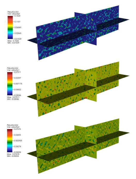
**Figure 11.** Steady-state flow through the packed cylinder geometry in Figure 7 (right). From top to bottom, we show the axial (x) and transverse (y) and (z) velocities. Inlet axial velocity is 0.01 cm/sec with Re = 0.5. Spheres have not been voided in the visualization unlike in Figures 9 and 10. Computation was performed on OLCF Titan using 131,072 processor cores.
