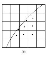
**Figure 4.** (a) Cell stencil showing sets of nearest neighbors. Neighbor cells with the same approximate distance to the center cell are indicated by a common number. (b) Interpolation from cell centroid data to cell center: Target point (the cell center) is shown with  $\times$  and support points are shown with  $\bullet$ . In this example only sets 1 and 2 of nearest neighbor cells are used.
