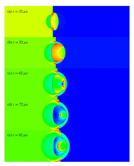
**Figure 15.** Density profiles of the shock-bubble test. The same color table as Figure 8 is used with limits (a)[0.997, 1.534], (b)[0.988, 1.607], (c)[0.999, 1.625], (d)[1.000, 1.623], and (e)[1.000, 1.646] for air and (a)[0.181, 0.221], (b)[0.178, 0.219], (c)[0.206, 0.221], (d)[0.215, 0.234], and (e)[0.218, 0.230] for helium.
