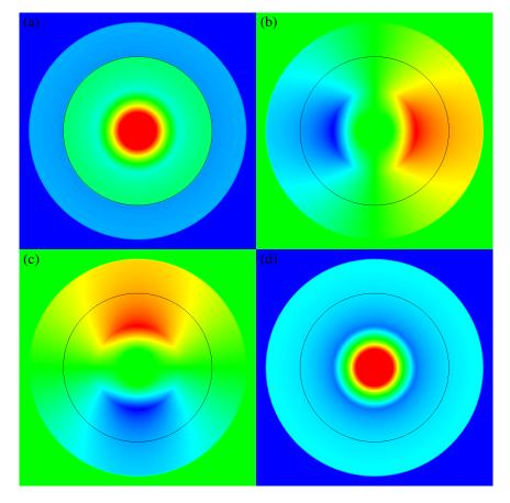
**Figure 9.** Results for 2-D Sod problem at finest resolution. (a) Density, (b) x-momentum, (c) y-momentum and (d) pressure. The same color table as Figure 8 is used with limits [1.0, 3.0] for density and pressure and [-0.614, 0.614] for momentum.
