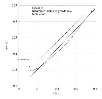
Figure 12. Amplitude of the perturbation on the front in the RMI simulation.
