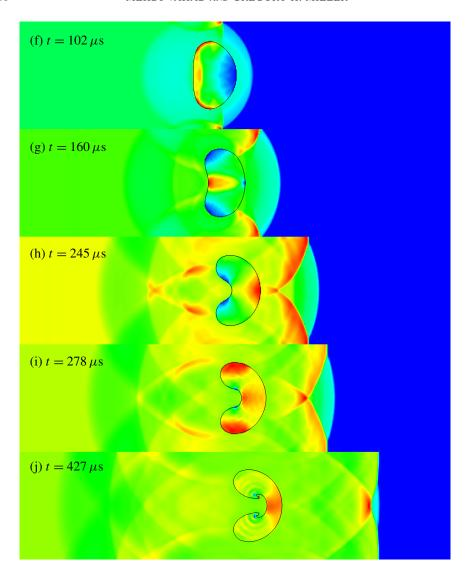
**Figure 15.** (continued) Density profiles of the shock-bubble test. The same color table as Figure 8 is used with limits (f)[1.000, 1.905], (g)[1.000, 1.664], (h)[1.000, 1.514], (i)[1.000, 1.554], and (j)[1.000, 1.584] for air and (f)[0.223, 0.231], (g)[0.231, 0.244], (h)[0.231, 0.238], (i)[0.230, 0.236], and (j)[0.229, 0.247] for helium.
