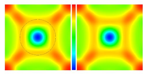
**Figure 8.** Density profile for smooth perturbation test at t = 0.6 on a 512  $\times$  512 grid. Left: dual gas simulation, front position shown with solid line. Right: result for single gas simulation with no front-tracking. The color table limits are [0.9, 1.04].
