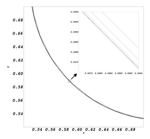
**Figure 6.** Final front position in the front advection problem. Inset: blowup of the front position. From right to left for h equal to  $\frac{1}{32}$ ,  $\frac{1}{64}$ ,  $\frac{1}{128}$ ,  $\frac{1}{256}$  and  $\frac{1}{512}$ .
