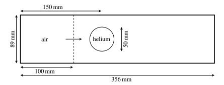
Figure 14. Initial configuration of the shock-bubble problem.
