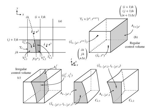
Figure 2. Geometry discretization and definitions.
