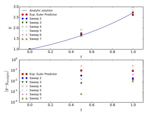
**Figure 8.** Effect of perturbation of the linear problem on SDC iteration convergence. Error is injected during Sweep 3 which results in an error larger than the initial predictor but is then damped by Sweeps 5 and 6.
