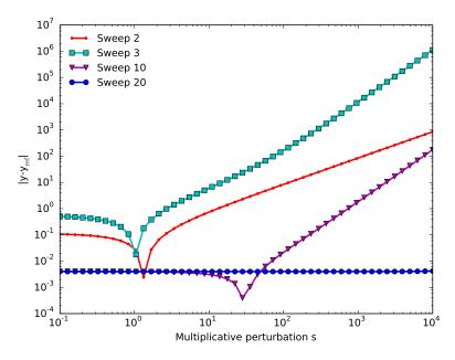
**Figure 9.** Effect of perturbation magnitude on SDC convergence rate. Reference solution  $y_{ref}$  is the analytic solution with s = 1.
