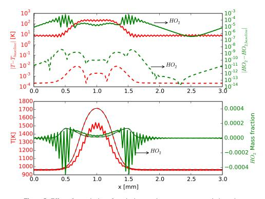
**Figure 5.** Effect of perturbation of continuity equation source term on solution using 6,4-RK and SDC integration schemes at time of baseline case ignition. Solid lines are the 6,4-RK solution, and dashed lines are the SDC solution for temperature (red) and HO<sub>2</sub> mass fraction (green). The upper plot shows the difference between the computed solution and the baseline while the lower plot shows the computed solution alongside the baseline (in solid black).
