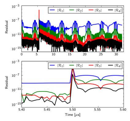
**Figure 6.** SDC residual response to soft perturbation for four correction sweeps given by  $\mathcal{R}_1$ - $\mathcal{R}_4$ . The lower plot is a zoom in on the region of the fault injection; note that the fault is clearly evident by examining the residual.
