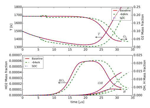
**Figure 4.** The effect of perturbation of the continuity equation source term on solution temporal evolution using 6,4-RK and SDC integration schemes; temporal plots were extracted at a fixed spatial location where error is injected. Notably, the SDC solution is indistinguishable from the baseline solution while the Runge–Kutta solution is silently and significantly corrupted.
