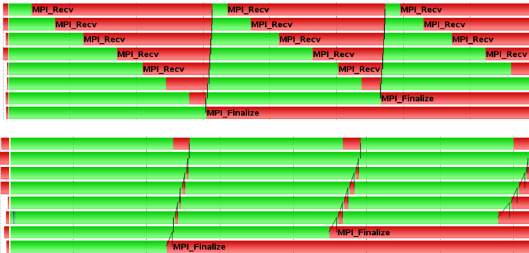
Figure 4. Vampir traces for the implementation \mathcal{P}_{m_0} with (N_{pr}, N_{it}) = (8, 3) for two different load balancing strategies. Top: Vampir trace for LB1. The Parareal runtime is R_{pa} = 7.964 s. Bottom: Vampir trace for LB2. The Parareal runtime is R_{pa} = 5.436 s.
