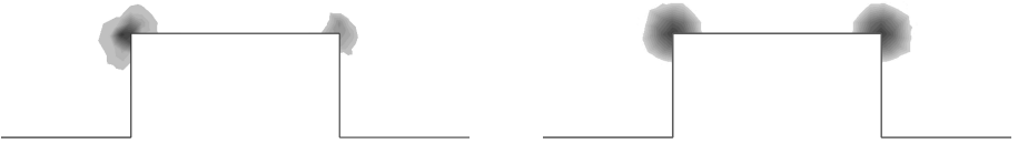
Figure 13. Weight functions on reentrant corners for the adaptive weight (left) and a priori weight (right). White regions represent w = 1 while darker regions are closer to w = 0 .
