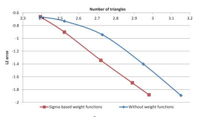
**Figure 4.** Log-log plot of  $L^2$  norm of error (with respect to control solution) as a function of the number of triangles, for  $b = \left(-\frac{1}{\sqrt{10}}, \frac{3}{\sqrt{10}}\right), g = 16x^2(1-x)^2, \varepsilon = 0.005$  (Example 1).
