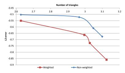
**Figure 9.** Comparison of weighted and nonweighted approaches for the Navier–Stokes example (log-log plot).
