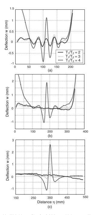
**Figure 11.** Wrinkle profiles for 0.025 mm thick, square Kapton<sup>®</sup> membrane at (a)  $\xi = 105$ , (b)  $\xi = 177$  and (c)  $\xi = 355$  mm for different load ratios.
