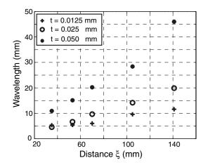
Figure 12. Average wrinkle wavelength in corner region of square membrane, vs. distance from corner, for  $T_1/T_2 = 1$ .
