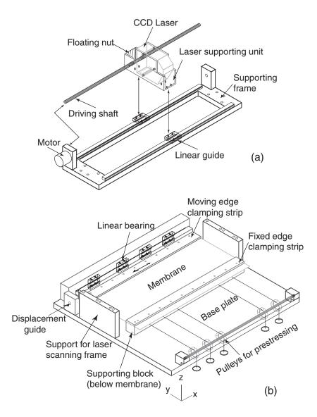
Figure 1. (a) Laser scanning frame, (b) Shear-rig.
