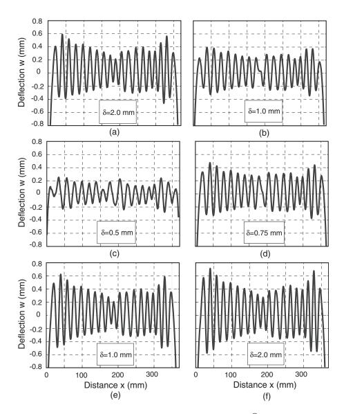
**Figure 5.** Section A-A of 0.025 mm thick Kapton<sup>®</sup> film under shear, during (a-c) unloading and (d-f) reloading.
