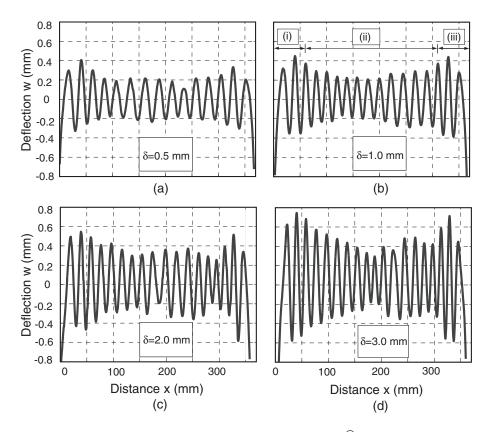
**Figure 4.** Section A-A of 0.025 mm thick Kapton<sup>®</sup> film for shear displacements of (a)  $\delta = 0.5$  mm, (b)  $\delta = 1.0$  mm, (c)  $\delta = 2.0$  mm, and (d)  $\delta = 3.0$  mm.
