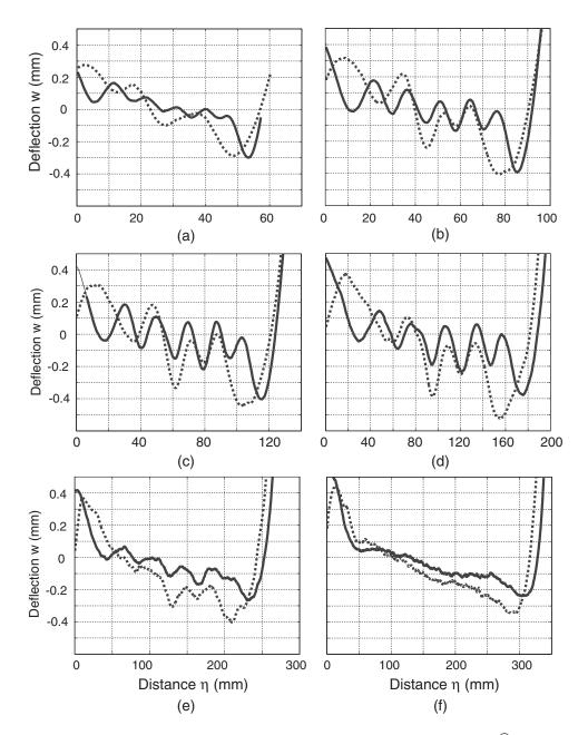
**Figure 9.** Wrinkle profiles in 0.025 mm thick, square Kapton<sup>®</sup> membrane, for  $T = T_1 = T_2 = 5$  N (dashed) and  $T = T_1 = T_2 = 20$  N (solid), at following distances from corner (a)  $\xi = 35$  mm, (b)  $\xi = 53$  mm, (c)  $\xi = 70$  mm, (d)  $\xi = 105$  mm, (e)  $\xi = 141$  mm and (f)  $\xi = 177$  mm.
