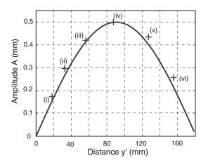
**Figure 7.** Comparison of longitudinal wrinkle profile with a sinusoidal mode shape, for sheared membrane.
