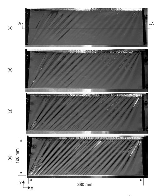
**Figure 3.** Wrinkle patterns for a 0.025 mm thick Kapton<sup>®</sup> film under shear displacements of (a)  $\delta = 0.5$  mm, (b)  $\delta = 1.0$  mm, (c)  $\delta = 2.0$  mm, and (d)  $\delta = 3.0$  mm.
