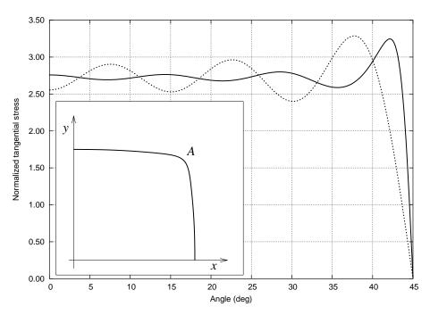
**Figure 3.** The tangential stress distribution along the  $\delta W$ -optimal hole shape (A) at N=23: Exact summation (the solid line) versus truncation (the dotted line)
