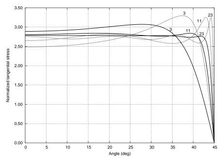
**Figure 5.** Tangential stress distribution along  $\mathcal{H}$ - and  $\delta W$ -optimal holes (solid and dotted lines, respectively) for N = 3, 11, 23.
