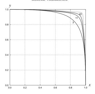
**Figure 4.** A quarter of the  $\mathcal{K}$ -optimal hole: evolution with increasing N (N = 3, 11, 22). The  $\delta W$ -optimal shape for N = 23 is added for comparison (dotted line).
