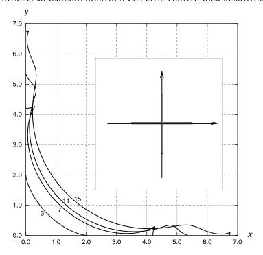
**Figure 6.** The energy-maximizing hole under square symmetry and remote shear: evolution to the limiting cross-like slit with increasing N. For N=3 we have a four-cusped hypocycloid (29).
