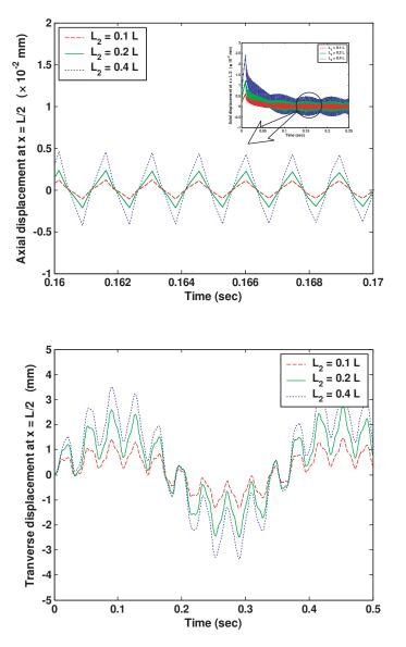
**Figure 12.** Axial and transverse displacements versus size of  $L_2$  on which thermal load is applied when c = 4 m/s.
