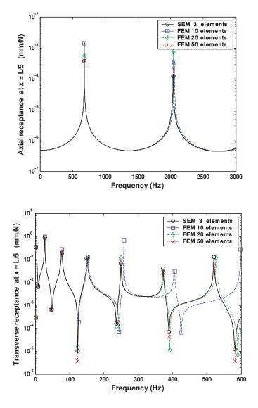
**Figure 8.** Comparison of the frequency response functions of the axial and transverse displacements obtained by the present SEM and FEM when c = 4 m/s and  $L_2 = 0.2L$ .
