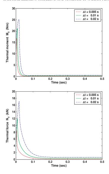
**Figure 14.** Time histories of the thermal moment  $M_T$  and thermal force  $N_T$  in the region  $L_1 \le x \le (L - L_2)$  versus duration of thermal load  $\Delta t$  when c = 4 m/s.
