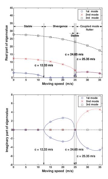
**Figure 4.** Moving speed dependence of the lowest first three eigenfrequencies of beam-plate.
