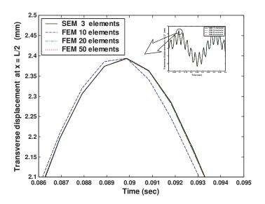
**Figure 9.** Comparison of the axial and transverse displacements obtained by the present SEM and FEM when c = 4 m/s and  $L_2 = 0.2L$ .
