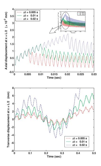
**Figure 15.** Time responses of axial and transverse displacements versus duration of thermal load  $\Delta t$  when c = 4 m/s.
