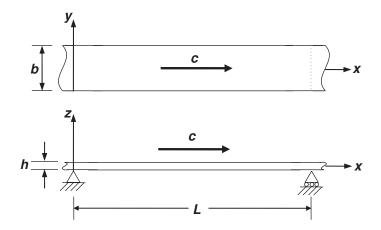
**Figure 1.** Geometry of an axially moving beam-plate.
