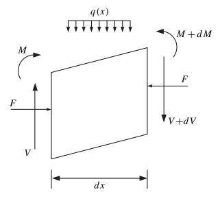
**Figure 1.** Free body diagram of a beam element.
