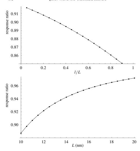
**Figure 2.** Small-scale effect versus location of the measurement (top) and length of CNT (bottom) for the model of a cantilevered CNT under distributed force.
