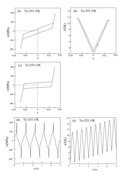
**Figure 2.** (a) The uniaxial stress-strain response in one cycle of SMA and, (b) the corresponding induced temperature deviation. (c) The corresponding uniaxial stress-strain response of SMA when the TMC is neglected. (d) The uniaxial stress-strain response in five cycles of SMA and (e) the corresponding induced temperature deviation. In all cases the reference temperature is  $T_0 = 253.15$  K.
