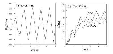
**Figure 7.** (a) The uniaxial response of the SMA/aluminum composite in 5 cycles loaded in the fibers direction and, (b) the resulting induced average temperature deviation at a reference temperature  $T_0 = 253.15$  K. Also shown is the corresponding induced temperature deviation in the unreinforced aluminum.
