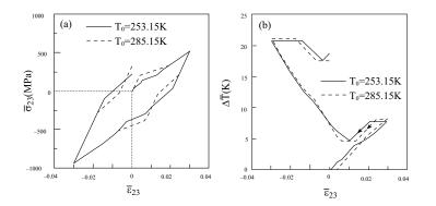
Figure 8. (a) The transverse shear stress-strain response in one cycle of the SMA/aluminum composite and, (b) the resulting induced average temperature deviation at reference temperatures:  $T_0 = 253.15$  K and 285.15 K.
