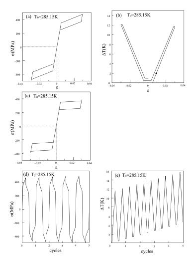
**Figure 3.** (a) The uniaxial stress-strain response in one cycle of SMA and, (b) the corresponding induced temperature deviation. (c) The corresponding uniaxial stress-strain response of SMA when the TMC is neglected. (d) The uniaxial stress-strain response in five cycles of SMA and (e) the corresponding induced temperature deviation. In all cases the reference temperature is  $T_0 = 285.15$  K.
