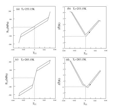
**Figure 9.** (a) The uniaxial stress-strain response in one cycle of the SMA/epoxy composite loaded in the fibers direction and, (b) the resulting induced average temperature deviation at a reference temperature  $T_0 = 253.15$  K. (c) The uniaxial stress-strain response in one cycle of the SMA/epoxy composite loaded in the fibers direction and, (d) the resulting induced average temperature deviation at a reference temperature  $T_0 = 285.15$  K.
