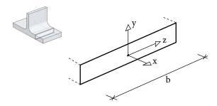
**Figure 8.** Flange cross sectional axis definitions.
