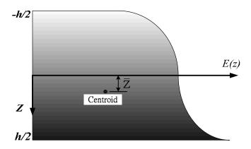
**Figure 4.** Distribution of the Young's modulus in the thickness direction of an FGM plate.
