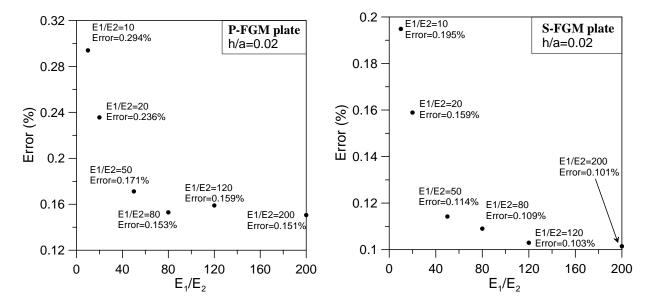
**Figure 14.** Error of maximum deflection of P-FGM plates versus ratio  $E_1/E_2$  between Young's moduli. Top: P-FGM plate; bottom: S-FGM plates. In both cases h/a = 0.02.
