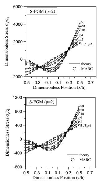
**Figure 10.** Distribution of stresses  $\sigma_x$  (top) and  $\sigma_y$  (bottom) at the center of an S-FGM plate along the thickness direction for different  $E_1/E_2$  ratios.
