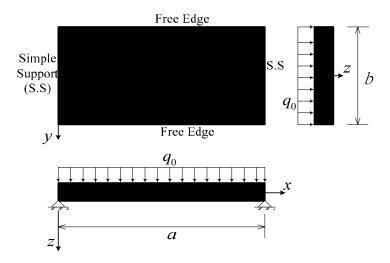
**Figure 1.** The configuration of an FGM plate.
