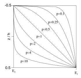
**Figure 2.** Variation of the Young's modulus of a P-FGM plate with differing material parameters *p*.
