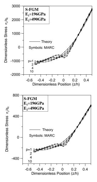
**Figure 11.** Distribution of stresses  $\sigma_x$  (top) and  $\sigma_y$  (bottom) at the center of an S-FGM plate along the thickness direction for differing material parameters  $p \ge 1$ .
