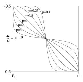
**Figure 3.** Variation of the Young's modulus of an S-FGM plate with differing material parameters *p*.
