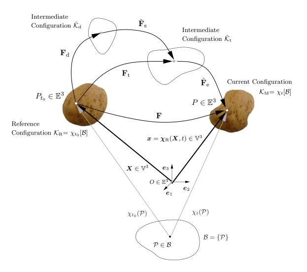
Figure 2. Reference, current, and intermediate configuration.
