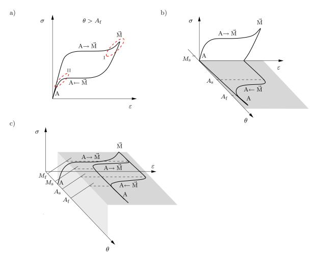
**Figure 1.** Sketch of the pseudoelasticity and the shape memory effects. A: austenite; M: oriented (detwinned) martensite.
