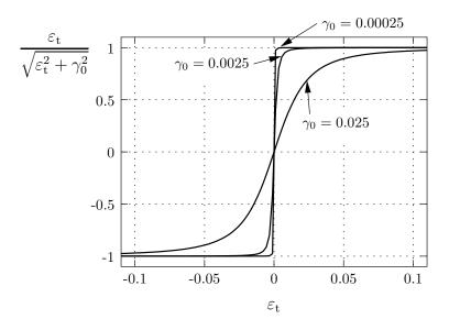
**Figure 3.** Illustration of  $\boldsymbol{e}_1 \cdot \mathbf{X}_{\theta} \boldsymbol{e}_1 \sim \varepsilon_t / \sqrt{\varepsilon_t^2 + \gamma_0^2}$  for uniaxial tension-compression load.
