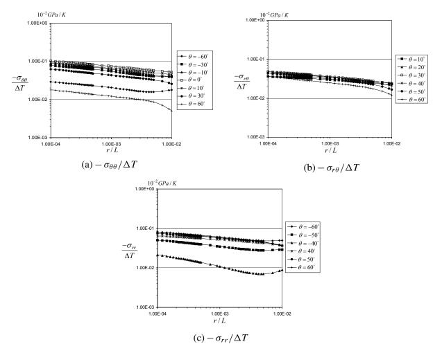
**Figure 10.** Stress distributions of  $-\sigma_{\theta\theta}/\Delta T$  for various angles of  $\theta$  ( $\alpha_{2D}=0.4, \beta_{2D}=0.2$ ).
