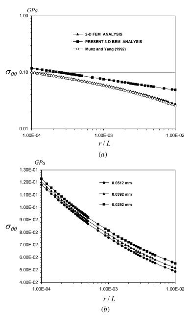
**Figure 6.** Stress distributions of  $\sigma_{\theta\theta}$  at the interface near the singular point on the stress singularity line for a uniform temperature variation ( $\Delta T = -100 \,\mathrm{K}$ ).
