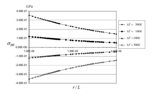
**Figure 7.** Stress distributions of  $\sigma_{\theta\theta}$  at the interface for various uniform temperature variations in a semilog scale.
