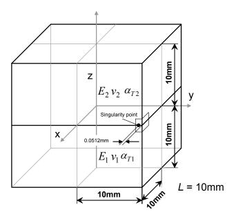
**Figure 4.** Model for analysis of a three-dimensional joint.
