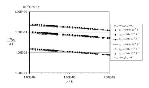
**Figure 11.** Effects of  $\alpha_{T2}$  ( $\alpha_{T1}1.0x10^{-6}K^{-1}$ ) on  $\sigma_{\theta\theta}/\Delta T$  at the interface  $\theta = 0$  for  $(\alpha_{2D} = 0.4, \beta_{2D} = 0.2)$  and  $(\alpha_{2D} = 0.3, \beta_{2D} = 0.2)$ .
