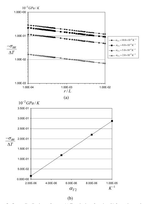
**Figure 9.** Stress distributions of  $-\sigma_{\theta\theta}/\Delta T$  at the interface  $\theta=0^{\circ}$  for various values of  $\alpha_{T2}$  ( $\alpha_{T1}=1.0x10^{-6}K^{-1}$  and  $\alpha_{2D}=0.6$ ,  $\beta_{2D}=0.2$ ).
