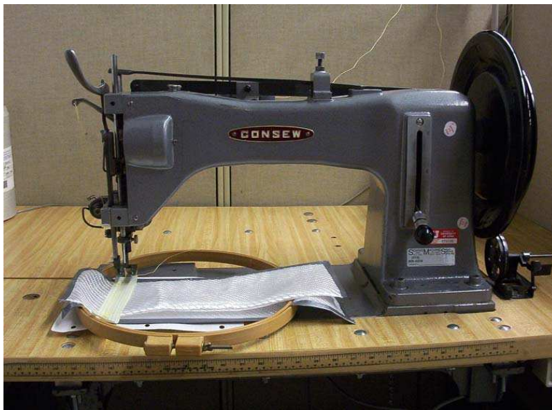
Figure 5. Sewing machine used to stitch, with Kevlar 29 thread, the plies of Dyneema inserted in the quilting hoop, with the aid of engineering paper. This process has also been used for the other materials discussed in the paper.
