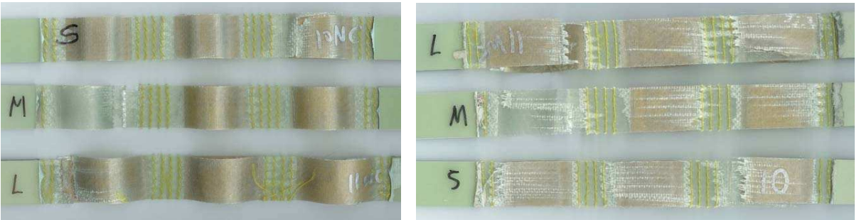
Figure 17. Top and bottom views of fractured main links and waiting links in E-glass specimens with small, medium and large round cores. Specimen width is 25.4 mm.
