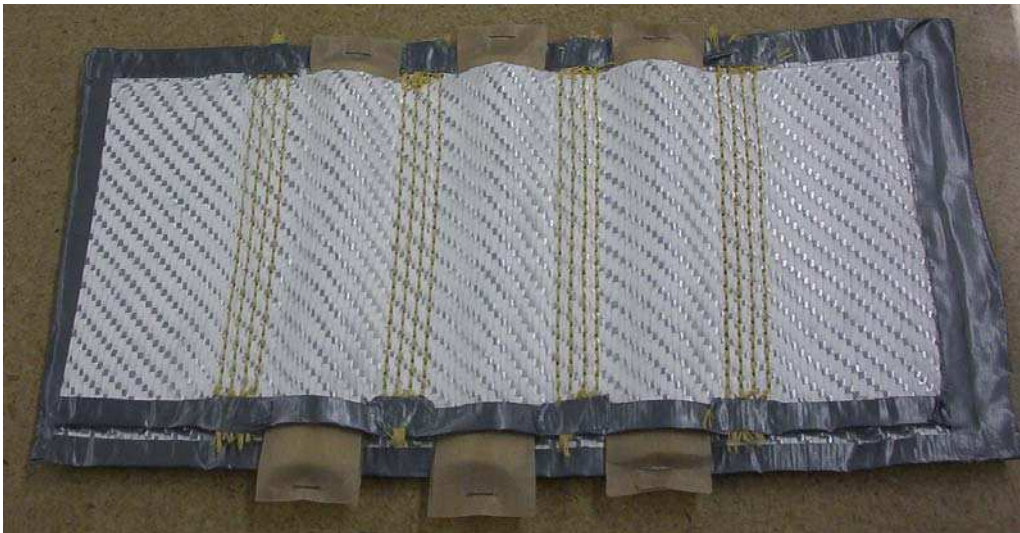
Figure 7. Dyneema specimen ready for resin infiltration.
