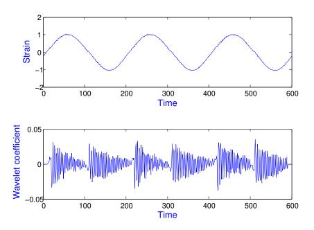
Figure 20. Strain and its wavelet transform; crack is 41%.
