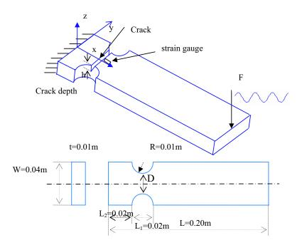
Figure 1. A cantilever beam with a crack.
