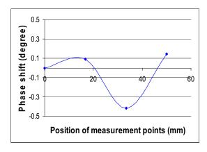
Figure 26. Phase shift distribution of the beam with crack of 58% depth.
