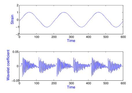
Figure 19. Strain and its wavelet transform; crack is 19%.
