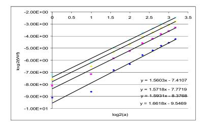
**Figure 6.** Maxima lines versus scale for five levels of crack: the lowest line is for the crack of 30% and the highest line is for the crack of 60%.
