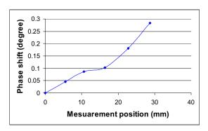
Figure 13. Phase shift distribution of the intact beam.
