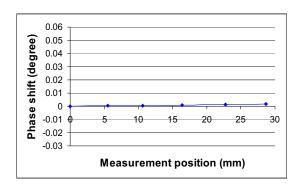
**Figure 9.** Phase shift distribution of the intact beam.
