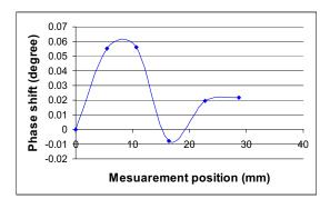
Figure 16. Phase shift distribution of the beam with crack of 60% depth.
