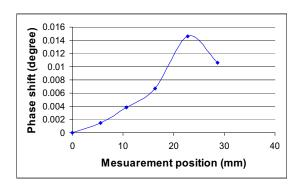
Figure 14. Phase shift distribution of the beam with crack of 20% depth.
