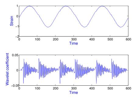
Figure 21. Strain and its wavelet transform; crack is 58%.
