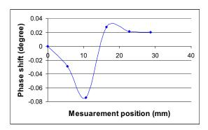
**Figure 15.** Phase shift distribution of the beam with crack of 40% depth.
