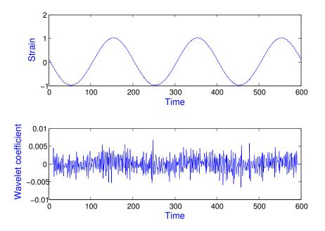
**Figure 18.** Strain and its wavelet transform; crack is 0%.
