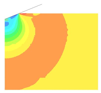
**Figure 20.** The first principal stress (in Pa) at indentation of a  $\Lambda(\epsilon_{\text{repr}} = 8\%) = 100$  material with hardening exponent n = 0.33 and representative stress  $\sigma(\epsilon_{\text{repr}} = 35\%) = 240$  MPa and interfacial friction  $\mu_i = 0.25$ .
