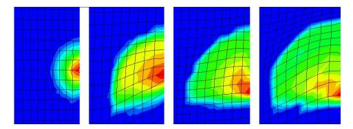
**Figure 5.** Contact pressure distribution at  $\Lambda = 1$ ,  $\Lambda = 10$ ,  $\Lambda = 100$  and  $\Lambda = 1000$ , for elastic perfectly plastic material. Only half of the contact region is visible in the figure. The scratch direction is upwards.
