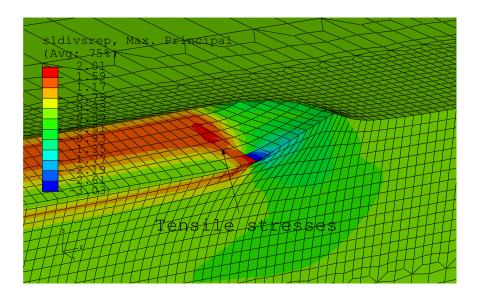
**Figure 18.** The first principal stress divided by the representative stress at scratching of a  $\Lambda(\epsilon_{\text{repr}} = 8\%) = 100$  material with hardening exponent n = 0.33, representative stress  $\sigma(\epsilon_{\text{repr}} = 35\%) = 240$  MPa and interfacial friction  $\mu_i = 0.25$ .
