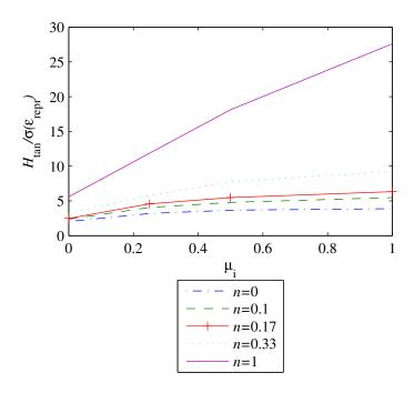
**Figure 11.** The influence of friction on tangential hardness for strain hardening materials with different hardening n. Simulations with  $\Lambda(\epsilon_{\text{repr}} = 8\%) = 100$ .
