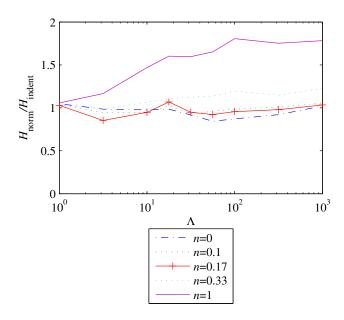
**Figure 15.** Ratio of scratch normal hardness to indentation hardness. Simulations with different n and  $\Lambda(\epsilon_{\text{repr}} = 8\%)$ .
