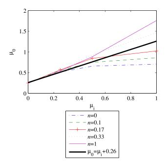
**Figure 14.** The apparent coefficient of friction  $\mu_0$  as a function of interfacial friction  $\mu_i$ . Simulated with n=0, n=0.1, n=0.17, n=0.33, n=1 and  $\Lambda(\epsilon_{\text{repr}}=8\%)=100$ . Equation (18) is plotted as a reference.
