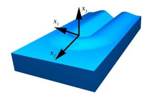
**Figure 3.** Cartesian coordinates  $x_i$  (following the tip of the stylus). Scratching is performed in the  $x_2$  direction.
