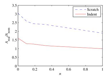
**Figure 6.** The actual normally projected contact area,  $A_{\text{real}}$ , divided by the nominal contact area,  $A_{\text{nom}}$ , plotted against the hardening parameter n. Results both for indentation and scratching.  $\Lambda(\epsilon_{\text{repr}} = 8\%) = 1000$ .
