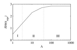
**Figure 2.** Sketch of the characteristic behavior of indentation hardness [Johnson 1985]. The indentation hardness H divided by the stress  $\sigma(\epsilon_{\text{repr}})$  is plotted against the nondimensional strain parameter  $\Lambda$ .
