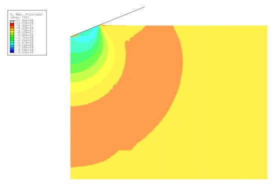
**Figure 19.** The first principal stress (in Pa) at frictionless indentation of a  $\Lambda(\epsilon_{\text{repr}} = 8\%) = 100$  material with hardening exponent n = 0.33 and representative stress  $\sigma(\epsilon_{\text{repr}} = 35\%) = 240$  MPa.
