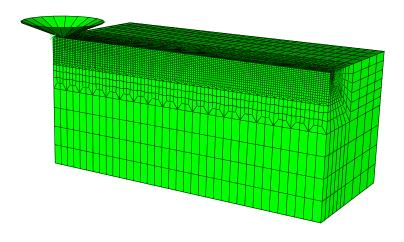
**Figure 4.** Finite elements mesh. Linear 8-node brick elements. Symmetry conditions apply to the surface in view. The stylus is also shown.
