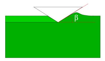
**Figure 1.** The angle  $\beta$  of a conical indenter/stylus.
