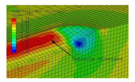
**Figure 17.** The first principal stress divided by the representative stress at frictionless scratching of a  $\Lambda(\epsilon_{\text{repr}} = 8\%) = 100$  material with hardening exponent n = 0.33 and representative stress  $\sigma(\epsilon_{\text{repr}} = 35\%) = 240$  MPa.
