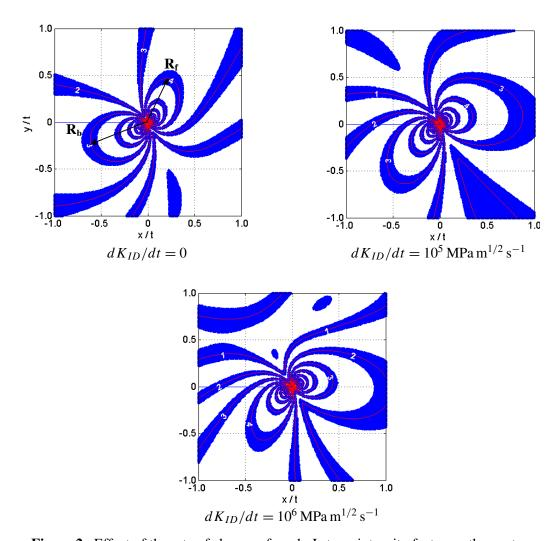
**Figure 2.** Effect of the rate of change of mode-I stress intensity factor on the contours of constant maximum shear stress around the crack tip in an FGM ( $\alpha = 0.57$ ,  $K_{ID}(t) = 1$  MPa m<sup>1/2</sup>,  $K_{IID}(t) = 1$  MPa m<sup>1/2</sup>, c = 650 ms<sup>-1</sup>, dc/dt = 0). The front and rear apogee radii are marked in part (a) with  $R_f$  and  $R_b$ , respectively.
