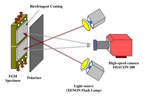
**Figure 6.** Photoelastic configuration for testing FGM specimens.
