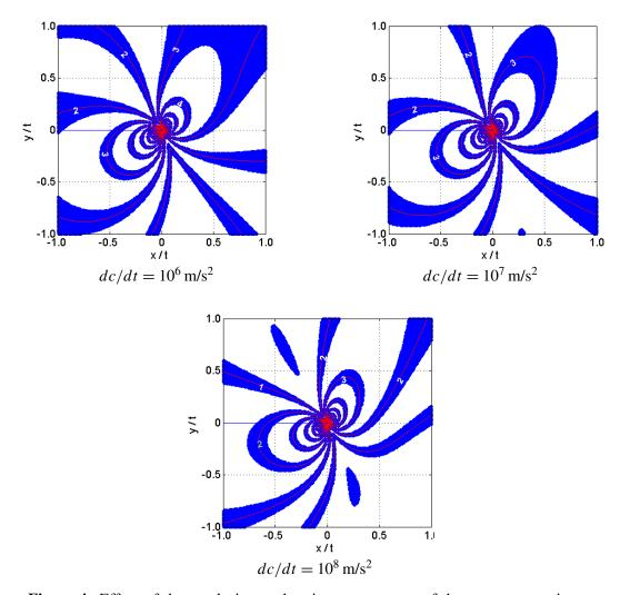
**Figure 4.** Effect of the crack tip acceleration on contours of the constant maximum shear stress around the crack tip in an FGM ( $\alpha = 0.57$ ,  $K_{ID}(t) = 1$  MPa m<sup>1/2</sup>,  $K_{IID}(t) = 1$  MPa m<sup>1/2</sup> $dK_{ID}(t)/dt = 0$ , c = 650 ms<sup>-1</sup>).
