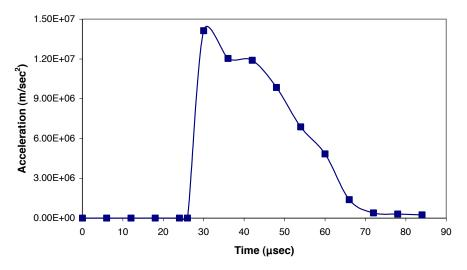
Figure 9. Crack tip acceleration as a function of time.
