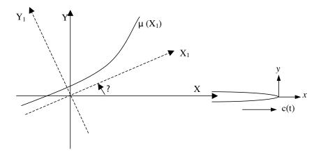
**Figure 1.** Propagating crack orientation with respect to the direction of property variation in a FGM.
