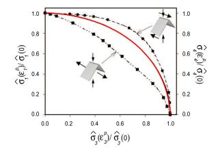
**Figure 3.** Initial yield surface of the folded plate core subject to two different combined loadings. The true stresses are normalized by the initial yield stress associated with each simple loading history under quasistatic loading. The solid line corresponds to the ellipsoidal yield surface invoked in the constitutive model when all the plastic Poisson ratios are taken to be zero. The folded core has the same geometrical parameter as that in Figure 2.
