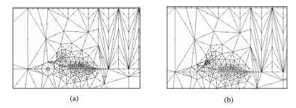
**Figure 6.** Element refinement at the crack tip for the SIF computation: (a) finer elements around the crack tip at the serration's bottom corner; (b) finer elements around the crack tip at the serration's peak.
