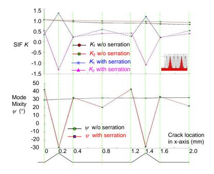
**Figure 13.** *K* and  $\psi$  vs crack location for sparse sharp serrations (80.5°).
