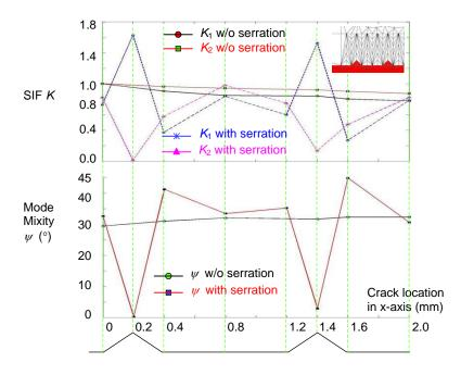
**Figure 8.** *K* and  $\psi$  versus crack location for sparse small serrations (45.0°).
