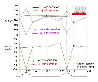
**Figure 10.** *K* and  $\psi$  vs crack location for sparse medium serrations (63.4°).
