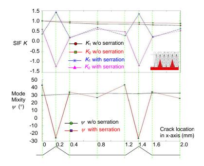
**Figure 12.** *K* and  $\psi$  vs crack location for sparse sharp serrations (76.0°).
