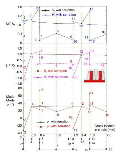
**Figure 14.** K and  $\psi$  vs crack location for sparse rectangular servations (90.0°).
