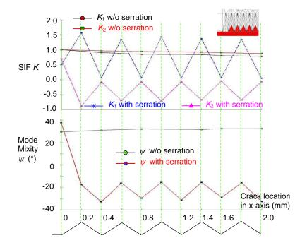
**Figure 11.** *K* and  $\psi$  vs crack location for dense medium serrations (63.4°).
