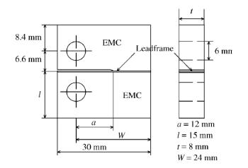
Figure 2. Geometry of DCB sandwich specimen.
