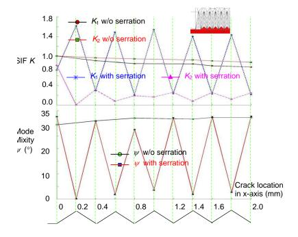
**Figure 9.** *K* and  $\psi$  versus crack location for dense small serrations (45.0°).
