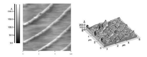
Figure 1. AFM images of a glass/epoxy interface crack.
