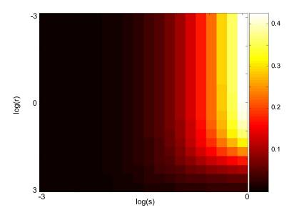
**Figure 3.** Overall transducer efficiency  $\eta$  as a function of the parameters *r* and *s* (log scales) when v = 0.3.
