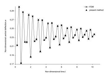
Figure 8. Damped response of a simple supported banana fiber reinforced square orthotropic plate for  $C_v = 1.25$ .
