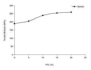
Figure 1. Effect of PCL content on tensile modulus of HDPE/PCL blend.
