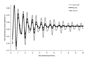
Figure 9. Damped response of a smiple supported banana fiber reinforced orthotropic plate for aspect ratio R = 1.
