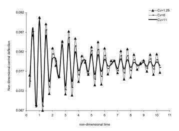
Figure 15. Damped response of a clamped supported banana fiber reinforced orthotropic plate for aspect ratio, R = 1.
