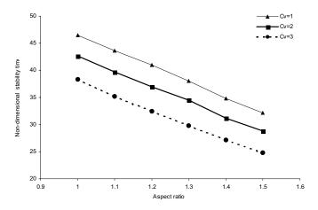
**Figure 12.** Nondimensional stability time at various aspect ratios for a simple supported banana fiber reinforced orthotropic plate.
