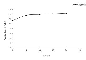
Figure 2. Effect of PCL content on tensile strength of HDPE/PCL blend.
