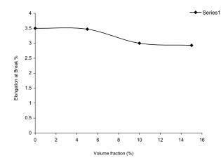
**Figure 6.** Effect of weight fraction of NaOH treated banana fibers on elongation at break of HDPE/PCL blend.
