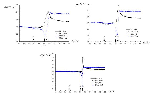
**Figure 2.** Transient response of a halfspace under a vertical disk load: horizontal (radial) and vertical at distances of 10 m (top left), 20 m (top right), and 100 m (bottom).
