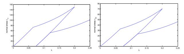
Figure 3. Biaxial extension of a material block: initial loading, unloading, and reloading.
