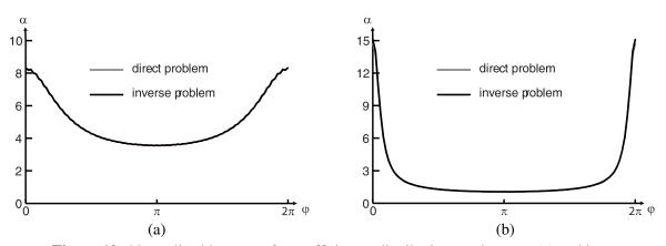
Figure 10. Normalized heat transfer coefficient  $\alpha$  distributions at the outer (a) and inner (b) boundaries for the direct and inverse problems.
