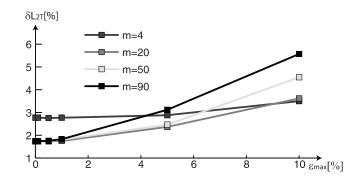
Figure 11. Dependence of relative error of temperature on maximal level of boundary condition disturbance for various numbers of the base functions smoothing the boundary conditions and the parameter f = 3.
