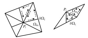
Figure 2. Neighbourhood  $\Omega_i$  of the  $P_i$  points inside (left) and outside (right) of the mesh.
