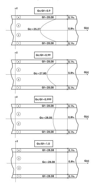
**Figure 5.** Assessment 3: Examples of different sandwich plates with core in FGM, following [Kashtalyan and Menshykova 2009].
