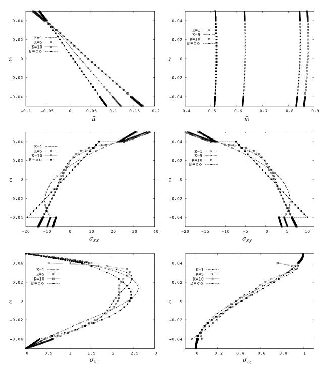
**Figure 10.** Benchmark: For the sandwich plate with core in FGM, displacements  $(\bar{u}, \bar{w}) = 10(u_x, u_z)E_ch^3/(\bar{p}_z a^4)$  and stresses  $\sigma_{xx}$ ,  $\sigma_{xy}$ ,  $\sigma_{xz}$  and  $\sigma_{zz}$  versus z for LD4 theory. In addition to the values  $\kappa = 1, 5, 10$  in Zenkour's formula (19), we consider an isotropic material with E = 225 GPa for the core ("E = co"). Thickness ratio: a/h = 10.
