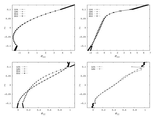
**Figure 9.** Benchmark: Sandwich plate with core in FGM. In-plane stress  $\sigma_{xx}$  (top row) and transverse-normal stress  $\sigma_{zz}$  (bottom row) versus z for  $\kappa = 1$  (left) and  $\kappa = 10$  (right). The thickness ratio is a/h = 4.
