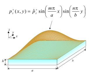
Figure 1. Notations and load configuration for the plates considered.
