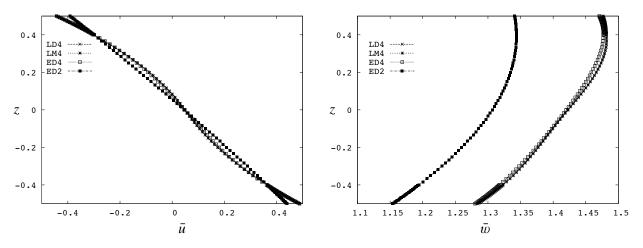
**Figure 6.** Assessment 3: Displacements  $\bar{u} = G_0 u_x / (\bar{p}_z h_0)$  and  $\bar{w} = G_0 u_z / (\bar{p}_z h_0)$  vs. *z*, for the sandwich plate with core in FGM proposed in [Kashtalyan and Menshykova 2009]. The shear modulus is  $G_c/G_f = 0.9$ .
