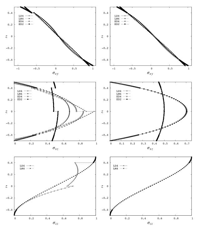
**Figure 7.** Assessment 3: Sandwich plates with core in FGM according to the solution and formula from [Kashtalyan and Menshykova 2009].  $G_c/G_f = 0.9$  (left column) and  $G_c/G_f = 0.999$  (right column).  $\sigma_{xy}$ ,  $\sigma_{xz}$  and  $\sigma_{zz}$  versus *z*.
