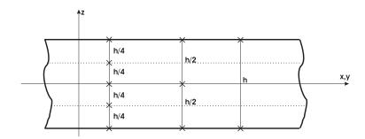
Figure 2. Assessment 1: Isotropic square plate with fictitious layers.
