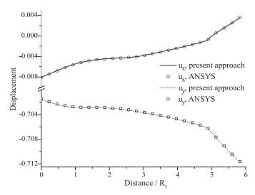
**Figure 4.** Variation of the displacements along the path  $(-3R_1, -5R_1) \div (0, 0)$  at time t = 8 sec.
