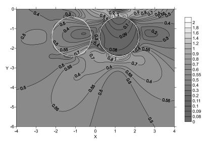
**Figure 13.** Contours of  $\tau_{\max}(z, t)/\sigma_0$  at time t = 0 sec.
