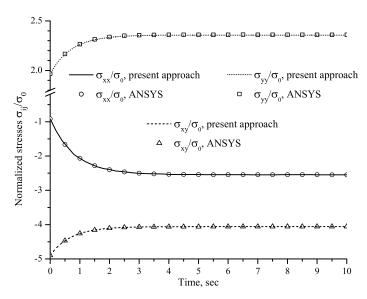
**Figure 6.** Variation of the normalized stresses at the point  $(-2.28R_1, -2.3R_1)$  located inside the viscoelastic matrix  $(N_{\text{St}} = 10)$ .
