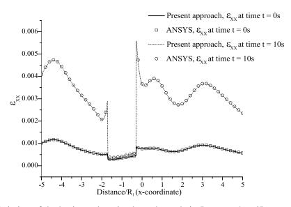
**Figure 5.** Variation of the horizontal strain along the path  $(-5R_1, -R_1) \div (5R_1, -R_1)$ .
