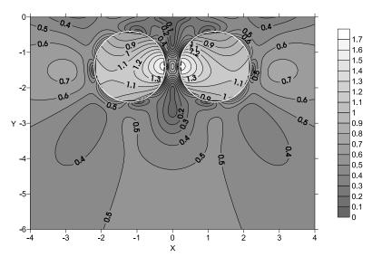
**Figure 15.** Contours of  $\tau_{\text{max}}(z, t)/\sigma_0$  at time  $t = 300 \,\text{sec}$ .
