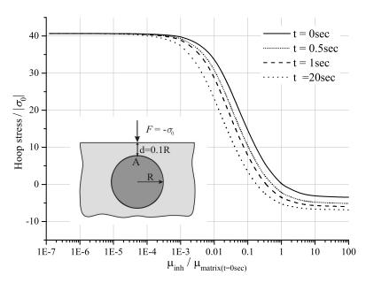
**Figure 9.** Variation of the normalized hoop stress at point A for loading case (ii).
