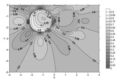
**Figure 14.** Contours of  $\tau_{\text{max}}(z,t)/\sigma_0$  at time t=5 sec.
