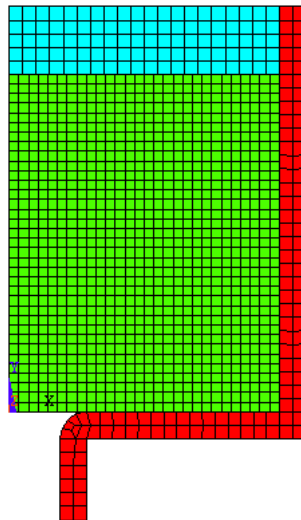
Figure 4. Initial finite element mesh for simulating the ram extrusion process with a die diameter of 15 mm.
