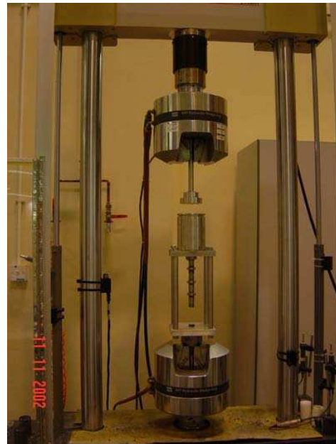
Figure 2. Experimental setup of the ram extrusion test: schematic diagram and laboratory apparatus.
