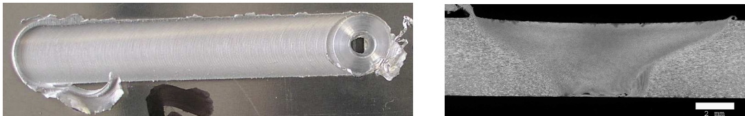
Figure 1. Top view of the weld (left) and cut orthogonal to the welding direction (right).
