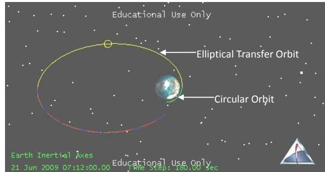
Figure 5. Satellites in the transfer elliptical orbit.
