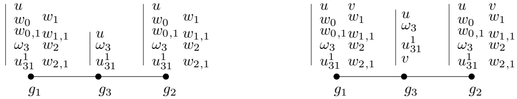
Figure 3. Description of the laminated beam finite element DOF. SinRef-6p (left) and SinRef-7p (right).
