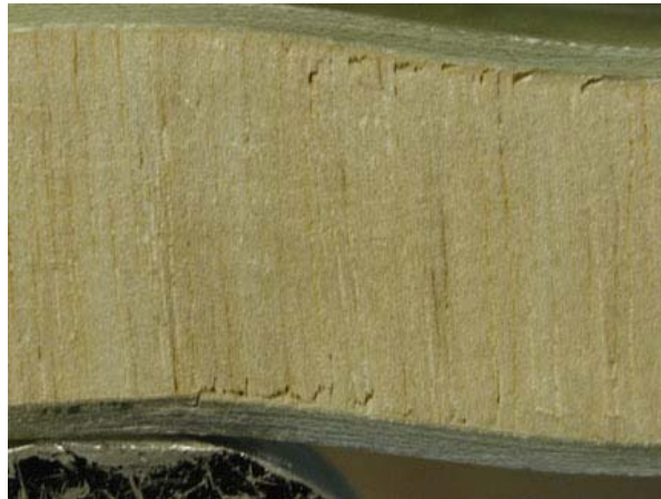
Figure 9. Cracking in balsa wood core of sandwich beam under three-point bending near support.
