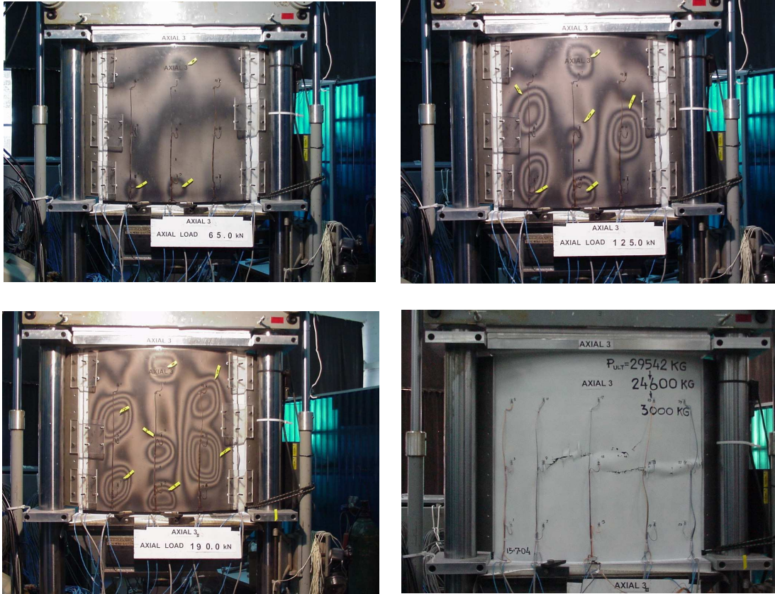
Figure 9. Panel AXIAL3: Development of the buckling pattern as a function of axial compression under 65 kN, 125 kN, 190 kN, and after collapse at 295.42 kN (bottom right).
