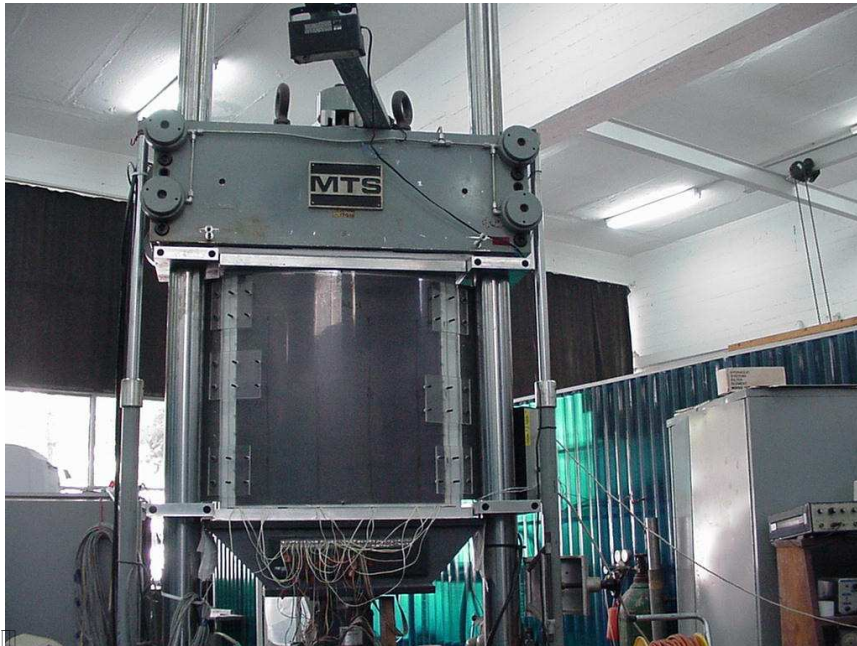
Figure 2. Panel in loading machine setup used at the Aerospace Structures Laboratory (ASL).
