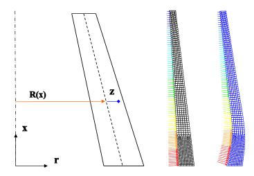
**Figure 1.** Shell geometry (left), loading (center), and deformation (right).
