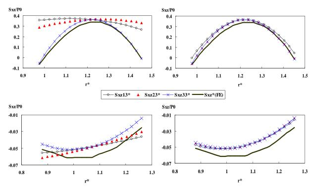
**Figure 10.** Comparison of different axial displacements on shear stress at  $x^* = 0.08$  (top) and  $x^* = 0.4$  (bottom), for  $Uz_3$  (left) and for  $Ux_3$  (right).
