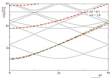
**Figure 5.** Dispersion curves in the wave number kd-frequency  $\omega d\sqrt{\rho/c_{44}^1}$  plane for the antisymmetric modes and l/d = 0.1 and a/d = 1.0; solid lines: thick plate with periodic cracks; dotted lines: thick plate with spring boundary conditions; dash-dotted lines: plate equation with spring boundary conditions.
