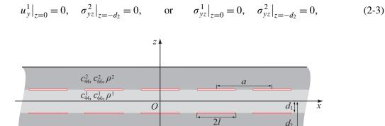
Figure 1. Elastic plate with periodic arrays of cracks.
