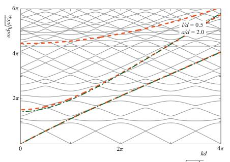
**Figure 6.** Dispersion curves in the wave number kd-frequency  $\omega d\sqrt{\rho/c_{44}^1}$  plane for the symmetric modes and l/d = 0.5 and a/d = 2.0; solid lines: thick plate with periodic cracks; dotted lines: thick plate with spring boundary conditions; dash-dotted lines: plate equation with spring boundary conditions.
