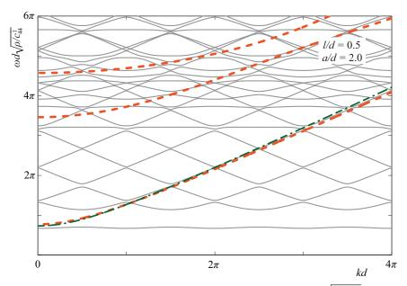
**Figure 7.** Dispersion curves in the wave number kd-frequency  $\omega d\sqrt{\rho/c_{44}^1}$  plane for the antisymmetric modes and l/d = 0.5 and a/d = 2.0; solid lines: thick plate with periodic cracks; dotted lines: thick plate with spring boundary conditions; dash-dotted lines: plate equation with spring boundary conditions.
