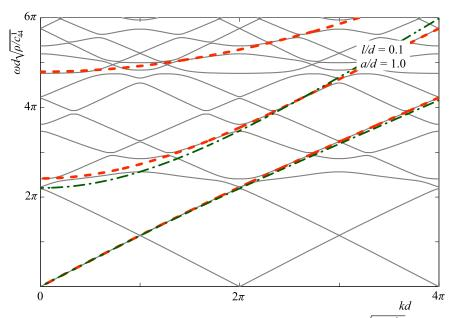
**Figure 4.** Dispersion curves in the wave number kd-frequency  $\omega d\sqrt{\rho/c_{44}^1}$  plane for the symmetric modes and l/d = 0.1 and a/d = 1.0; solid lines: thick plate with periodic cracks; dotted lines: thick plate with spring boundary conditions; dash-dotted lines: plate equation with spring boundary conditions.
