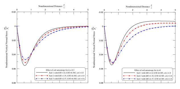
**Figure 3.** Effect of ratio E/E' on the vertical normal stress  $(\sigma_{zz})$  induced by a horizontal line load  $(P_x)$  when kz = -0.3 (left) and kz = 0 (right). Comparison of soils 1, 2, and 3.
