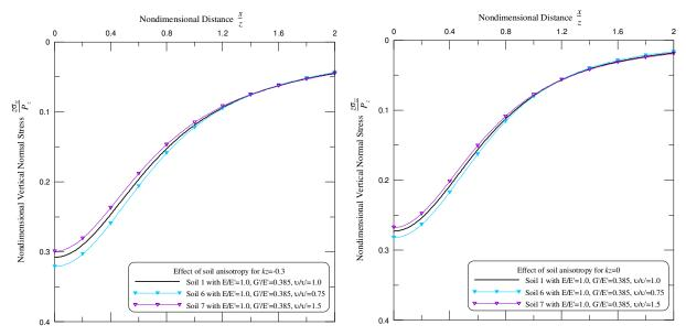
**Figure 9.** Effect of ratio v/v' on the vertical normal stress  $(\sigma_{zz})$  induced by a vertical line load  $(P_z)$  when kz = -0.3 (left) and kz = 0 (right). Comparison of soils 1, 6, and 7.
