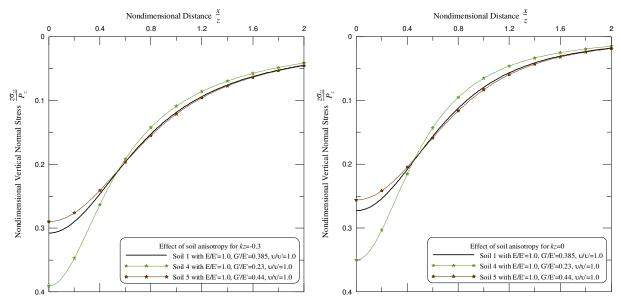
**Figure 8.** Effect of ratio G'/E' on the vertical normal stress  $(\sigma_{zz})$  induced by a vertical line load  $(P_z)$  when kz = -0.3 (left) and kz = 0 (right). Comparison of soils 1, 4, and 5.
