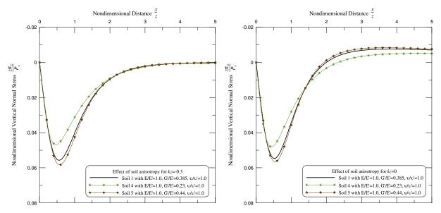
**Figure 4.** Effect of ratio G'/E' on the vertical normal stress  $(\sigma_{zz})$  induced by a horizontal line load  $(P_x)$  when kz = -0.3 (left) and kz = 0 (right). Comparison of soils 1, 4, and 5.
