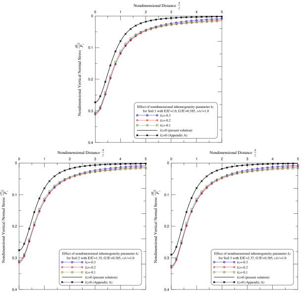
**Figure 6.** Effect of the inhomogeneity parameter kz on the vertical normal stress  $(\sigma_{zz})$  induced by a vertical line load  $(P_z)$  for soil types 1–3. (Continued on next page.)
