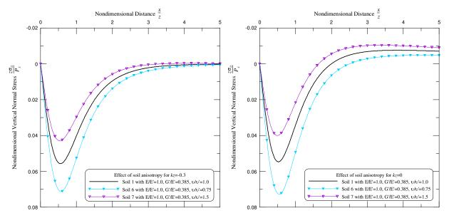
**Figure 5.** Effect of ratio v/v' on the vertical normal stress  $(\sigma_{zz})$  induced by a horizontal line load  $(P_x)$  when kz = -0.3 (left) and kz = 0 (right). Comparison of soils 1, 6, and 7.
