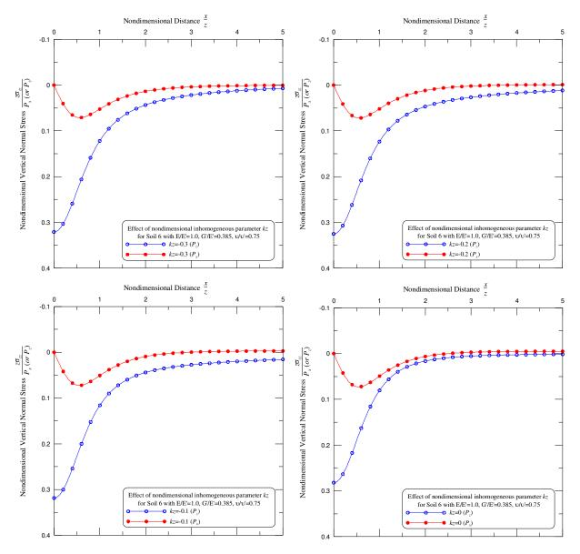
**Figure 10.** Effect of loading types  $(P_x \text{ and } P_z)$  on the vertical normal stress  $(\sigma_{zz})$  for cross-anisotropic soil 6 for kz = -0.3 (top left), -0.2, -0.1, and 0 (bottom right).
