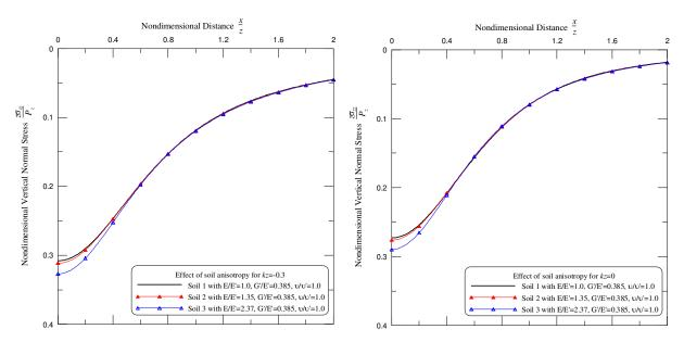
**Figure 7.** Effect of ratio E/E' on the vertical normal stress  $(\sigma_{zz})$  induced by a vertical line load  $(P_z)$  when kz = -0.3 (left) and kz = 0 (right). Comparison of soils 1, 2, and 3.
