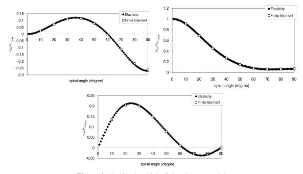
**Figure 4.** Verification of the finite element model.
