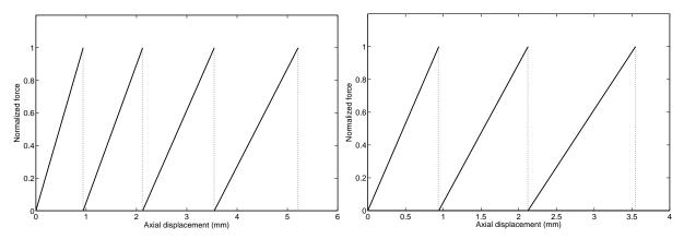
**Figure 17.** Force-displacement diagram for random breakages: three breakages (left) and two breakages (right).
