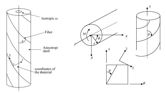
Figure 3. Helicoidal structure and its coordinate system.
