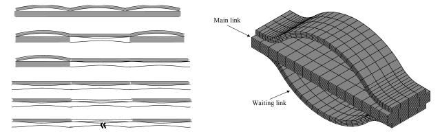
**Figure 1.** Left: A chain of bistable structures and their damage process. Gray regions represent the undamaged main strips. The broken main strips are shown in white. Right: A bistable structure with a symmetric waiting element.
