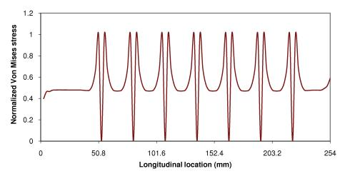
**Figure 7.** Stress distribution when the breakage locations are 50.8 mm apart  $(60^{\circ})$ .
