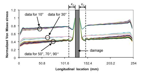
**Figure 6.** Normalized von Mises stress around the breakage.
