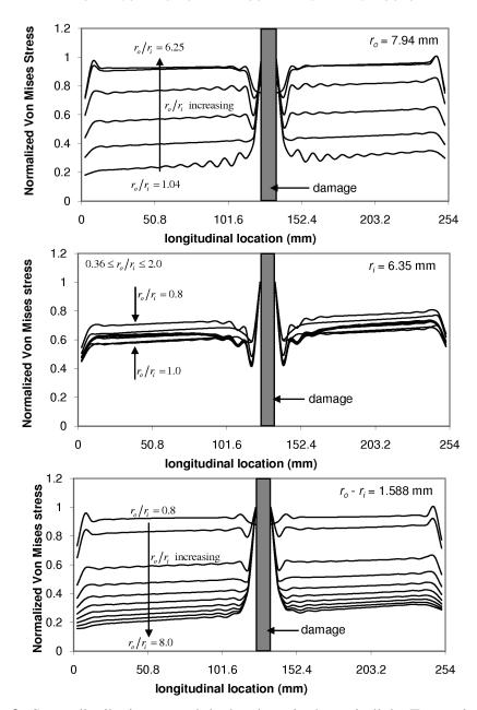
**Figure 9.** Stress distribution around the breakage in the main link. Top:  $r_i$  is varied while  $r_o$  remains at 7.94 mm. Middle:  $r_o$  is varied while  $r_i$  remains at 6.35 mm. Bottom:  $r_i$  and  $r_o$  are varied while the thickness of the waiting link is held at 1.59 mm.
