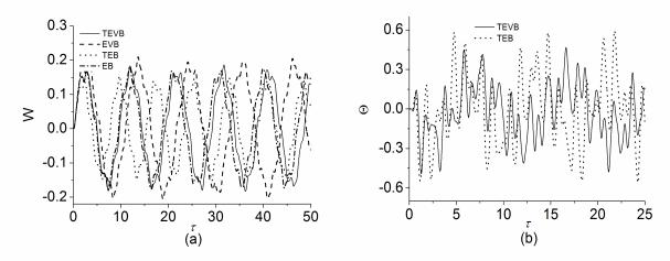
**Figure 10.** Time-history curves of the beams deflection W and thermal moment  $\Theta$ .
