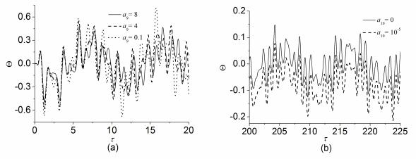
**Figure 12.** Time-history curves of thermal moment of TEVB, for various values of  $a_9$  (left) and  $a_{10}$  (right).
