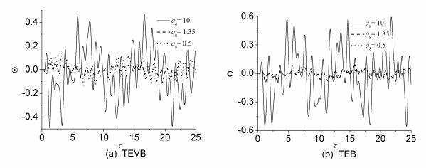
Figure 11. Time-history curves of the thermal moment of TEVB and TEB, for various values of  $a_8$ .
