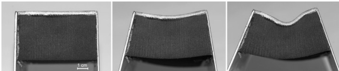
Figure 4. Progressive bending of a two-layer rubber block (undeformed configuration is shown on the left, a bent configuration in the center), evidencing bifurcation with long-wavelength bifurcation modes (shown on the right). Stiffness and thickness ratios between layers are (2.687 N/mm 2 )/(0.095 N/mm 2 ) and (3 mm)/(40 mm), respectively. The stiff layer (64.5 mm \times 3 mm \times 150 mm, made up of natural rubber, marked with a white pencil on the sample) is at the compressive side and coats a neoprene layer (64.5 mm \times 40 mm \times 150 mm).
