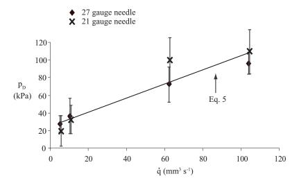
**Figure 8.** The mean pressure  $p_d \pm$  s.d. versus volumetric flow rate  $\dot{q}$  for the injection of PBS into adipose tissue using a 27 gauge needle and a 21 gauge needle. A least squares regression fit overlays the data.
