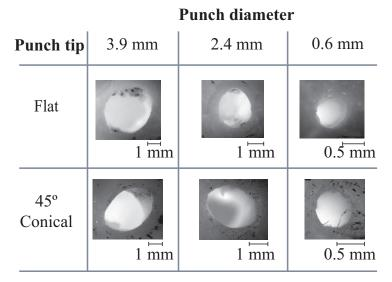
**Figure 2.** Images of the puncture site at the tissue surface following puncture by a range of metal punches of varying headshape at  $0.1 \text{ mm s}^{-1}$ .
