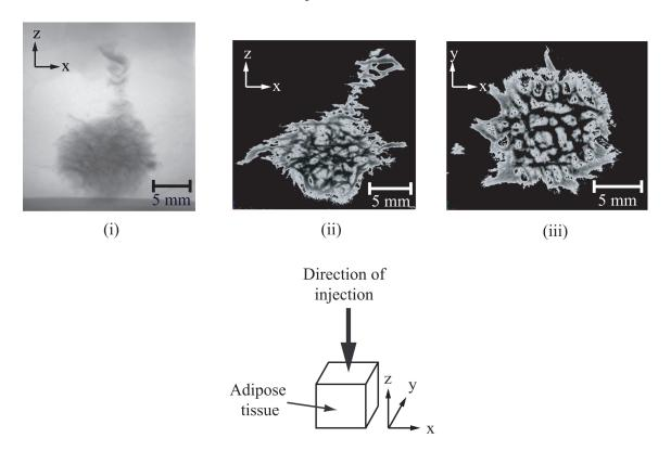
**Figure 9.** X-ray images of injection of 0.5 ml radio opaque dye (150 Urografin) into porcine adipose tissue by a hypodermic needle and syringe. Image (i) is a composite x-ray image. Images (ii) and (iii) are cross sections from a 3D reconstruction of 720 images taken at 0.5° around 360° of the sample.
