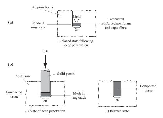
**Figure 5.** Sketches of (a) the hole formation in adipose tissue following deep penetration by a flat tipped or 45° conical tipped punch, and (b) the hole formation of the Shergold-Fleck ring-crack model.
