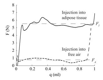
**Figure 7.** Force F versus the volume of saline injected q using a 0.4 mm diameter hypodermic syringe with a cross head displacement rate of 0.1 mm s<sup>-1</sup>.
