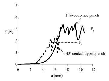
**Figure 1.** Force F versus displacement u for the penetration of porcine adipose tissue with 0.6 mm diameter metal punches with either a flat-bottom (solid line) or a 45° conical tip (dashed line). The displacement rate was 0.1 mm s<sup>-1</sup>.
