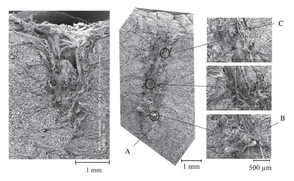
**Figure 3.** SEM images of the fracture surface of adipose tissue punctured by two punches of diameter 2.4 mm and tip geometry. Left: 45° conical tipped. Middle and right: flat-bottomed (A: compacted interlobular septa and reinforced basement membrane; B: interlobular septa fibres; C: reinforced basement membrane surrounding an adipocyte.
