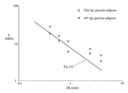
**Figure 4.** Comparison of the average pressure p required to penetrate adipose tissue with a range of solid punches of varying headshape. A prediction is shown for the pressure required to puncture adipose tissue with a flat tipped punch calculated from (3). The following parameter values were used in the calculations:  $J_C = 4.1 \,\mathrm{kJ}\,\mathrm{m}^{-2}$ , b/R = 0.5, a/R = 0.8,  $\mu = E/3 = 0.3 \,\mathrm{kPa}$ .
