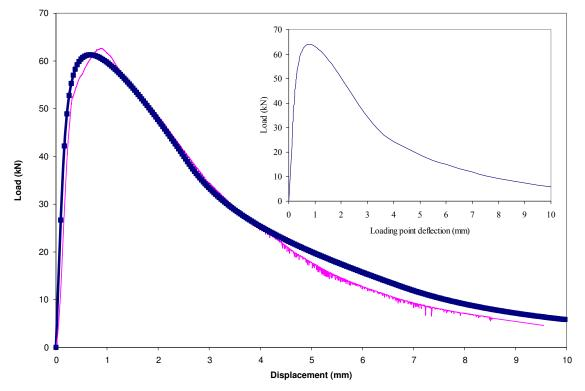
**Figure 3.** Large graph: load-deflection curves from experiments (thin curve) compared with an approximate method (thick curve/squares) in which the cohesive zone is regarded as a "hinge" in the central plane. Inset: load-deflection curve from the XFEM simulation. The agreement with the experimental curve is excellent both in terms of the shape and the maximum load carrying capacity.
