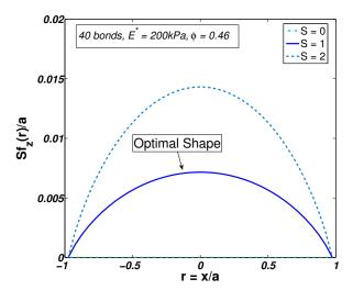
**Figure 2.** Schematic of a focal adhesion surface containing 40 bonds, having a system stiffness of  $E^* = 200 \,\mathrm{kPa}$ , and a tensile load factor of  $\varphi = 0.46$ . The surface shapes represented are for the following shape factors: S = 0 corresponding to adhesion between conforming surfaces, S = 1 corresponding to the optimal shape, and S = 2 corresponding to an overly curved focal adhesion surface in comparison to the optimal case.
