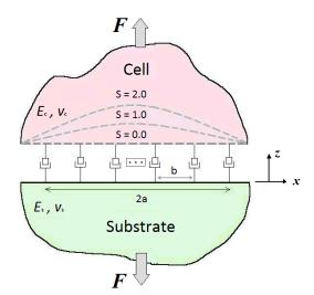
**Figure 1.** Idealized model of a single focal adhesion between a cell and substrate undergoing tensile loading. The cell and substrate are bonded together by an array of ligand/receptor bonds. The contact surface shapes of the focal adhesion are determined by a shape factor S which ranges in [0, 2], where S = 1 corresponds to the optimal contact shape for an initial uniformly loaded bond cluster.
