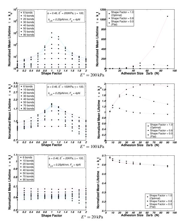
**Figure 3.** Effects of varying surface shape as defined by numerical shape factor values ranging within [0,2] on focal adhesion lifetime for different focal adhesion sizes ranging from 6 to 90 individual bonds. From top to bottom,  $E^* = 200 \,\mathrm{kPa}$ ,  $100 \,\mathrm{kPa}$ ,  $20 \,\mathrm{kPa}$ .
