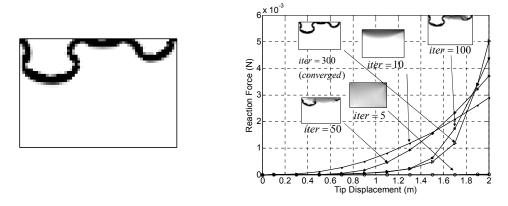
**Figure 11.** Optimized results by the developed method in recovering the reference layout exhibiting the nonlinear load-displacement curve in Figure 10. Left: the optimized layout. Right: load-displacement curves of the intermediate and final layouts.
