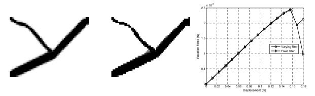
**Figure 7.** Layout optimization following the specific target reference points in the load-displacement trajectory: optimized layouts using fixed filter (left) and varying filter (middle); load-displacement trajectories for the optimized layouts (right).
