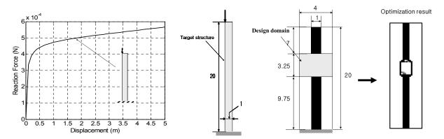
**Figure 16.** Example 5: a column design exhibiting geometrically weakening. Left: target trajectory. Middle: reference solid column structure ( $E=1~\text{N/m}^2$ ,  $\nu=0.3$ ). Right: an optimized layout in the expanded middle design domain.
