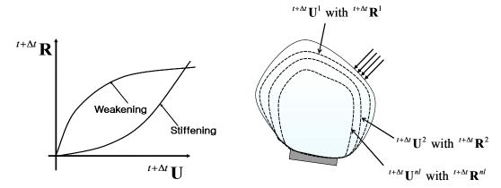
**Figure 1.** Geometric hardening or weakening model depicted with a displacement controlled Newton–Raphson scheme. (The prescribed displacement and the reaction force of the *i*-th load step are denoted by  $^{t+\Delta t}U^i$  and  $^{t+\Delta t}R^i$ , respectively. The number of load steps is nl).
