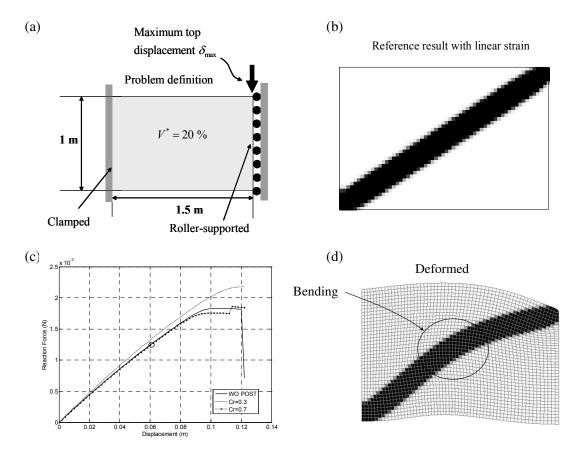
**Figure 6.** A test problem. (a) Problem definition (E=1 N/m<sup>2</sup>,  $\nu = 0.4$ ). (b) Optimized layout for  $V^* = 20\%$  when linear analysis is used. (c) Load-displacement trajectory of the layout in (b) by geometrically nonlinear analysis; Cr is the threshold design variable value for hard-kill postprocessing. (d) Deformed shape by nonlinear analysis when the top displacement reaches 0.12 m.
