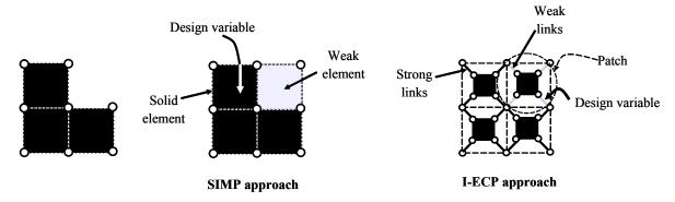
**Figure 2.** A structure (left) modeled with the SIMP (solid isotropic with penalization) method (middle) and the ECP-based method (right). All links have zero length.
