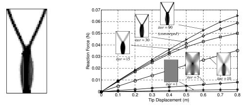
**Figure 13.** Iteration history of the load-displacement trajectories. The design objective is to find the target layout in Figure 12d.
