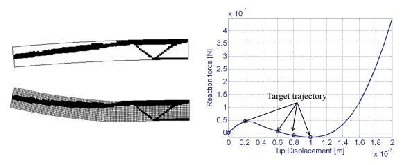
**Figure 15.** Example 4: a problem involving snap-through. Top left: optimized layout (undeformed). Bottom left: deformed shape (input displacement = 0.001). Right: load-displacement trajectory by the optimized layout; circles represent the target points.
