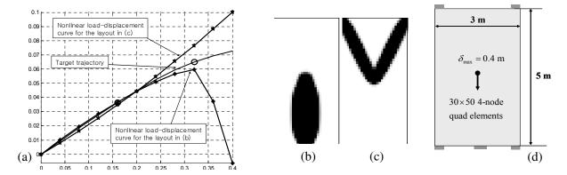
**Figure 12.** A problem to find a target nonlinear load-displacement trajectory. Left: target and limiting trajectories. Middle: reference layouts yielding linear and nonlinear limiting trajectories. Right: a compliance minimization problem used to obtain the given layouts with  $E = 1 \text{ N/m}^2$ , v = 0.4, volume = 20%.
