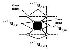
**Figure 3.** The e-th patch surrounding the e-th element for the ECP method. The inner nodes are the nodes defining the element while the outer nodes defining the e-th patch are used to connect patches sharing the same outer nodes. The solid lines connecting the inner and outer nodes denote zero-length one-dimensional elastic links.
