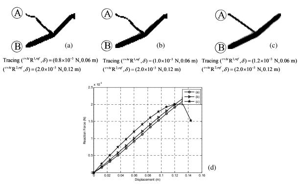
**Figure 8.** Top: optimized layouts following different target reference points in the load-displacement trajectory. Bottom: corresponding load-displacement trajectories.
