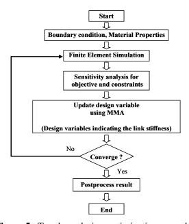
Figure 5. Topology design optimization procedure.
