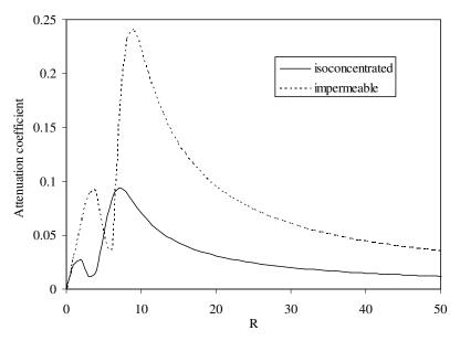
Figure 11. Attenuation coefficient versus *R* in semiconductor halfspace.
