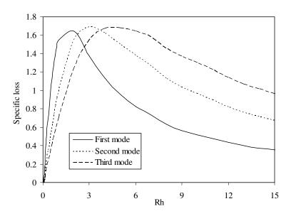
Figure 7. Specific loss versus *Rh* for PZT-Ge composite.
