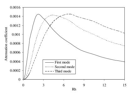
Figure 5. Attenuation coefficient versus Rh for PZT-Ge composite.
