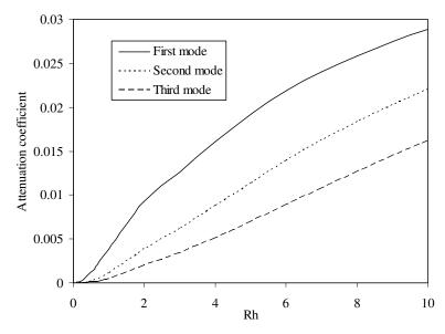
Figure 4. Attenuation coefficient versus Rh for CdSe-Ge composite.
