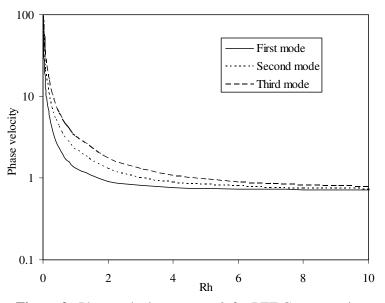
Figure 3. Phase velocity versus Rh for PZT-Ge composite.
