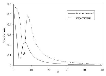
Figure 12. Specific loss versus *R* in semiconductor halfspace.
