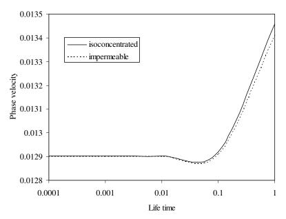
Figure 13. Phase velocity versus lifetime (in ps) of carrier field in semiconductor halfspace.
