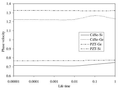
Figure 8. Phase velocity versus lifetime (in ps) of carrier field.
