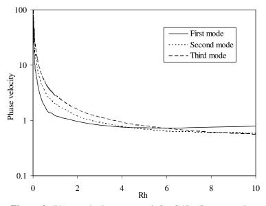
Figure 2. Phase velocity versus Rh for CdSe-Ge composite.
