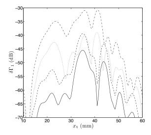
**Figure 2.** Signal response  $(\delta\Gamma_1)$  as a function of the position  $(x_t)$  of a 2 MHz transmitter for different sizes of the crack,  $2 \times 2 \text{ mm}$  (solid),  $2 \times 4 \text{ mm}$  (dashed),  $3 \times 3 \text{ mm}$  (dotted), and  $3 \times 6 \text{ mm}$  (dash-dotted).
