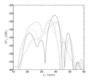
**Figure 5.** Signal response  $(\delta \Gamma_1)$  as a function of the position  $(x_t)$  of a 2 MHz transmitter for various values of the orientation of the crack,  $\varphi = 0$  (horizontal crack, solid),  $\varphi = 45^{\circ}$  (dashed),  $\varphi = 90^{\circ}$  (vertical crack, dotted),  $\varphi = 135^{\circ}$  (dash-dotted).
