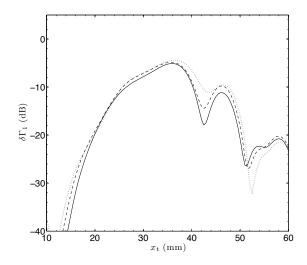
**Figure 6.** Signal response  $(\delta\Gamma_1)$  as a function of the position  $(x_t)$  of a 1 MHz transmitter for various values of the amplitude of the interface, b = 0 (solid), b = 0.5 mm (dashed), b = 1 mm (dotted).
