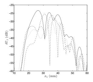
**Figure 4.** Signal response  $(\delta\Gamma_1)$  as a function of the position  $(x_t)$  of a 2 MHz transmitter for various values of the position of the crack relative to the corrugated interface,  $a_c = 1.25 \text{ mm}$  (solid),  $a_c = 2.5 \text{ mm}$  (dashed),  $a_c = 3.75 \text{ mm}$  (dotted),  $a_c = 0$  (dash-dotted).
