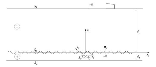
Figure 1. The geometry of a plate with a crack inside a cladding.
