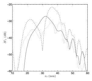
**Figure 3.** Signal response  $(\delta\Gamma_1)$  as a function of the position  $(x_t)$  of a 2 MHz transmitter for various values of the amplitude of the interface, b = 0 (solid), b = 0.5 mm (dashed), b = 1 mm (dotted).
