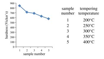
Figure 4. Effect of tempering temperature on hardness.
