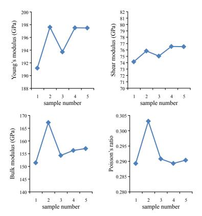
**Figure 6.** Effect of tempering temperature on elastic constants. Top: Young's modulus and shear modulus. Bottom: bulk modulus and Poisson's ratio.
