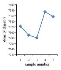
Figure 7. Effect of tempering temperature on density.
