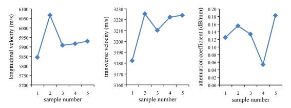
**Figure 5.** Effect of tempering temperature on ultrasonic properties. From left to right, longitudinal wave velocity, transverse wave velocity, and attenuation coefficient.
