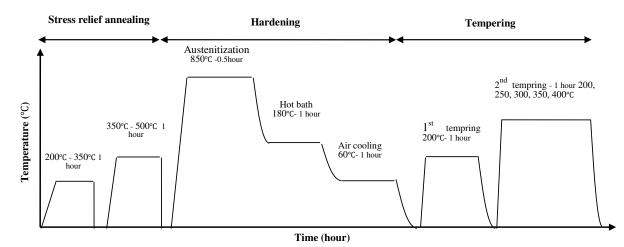
Figure 1. Heat treatment processes.
