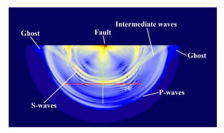
**Figure 2.** A two-dimensional numerical simulation of an earthquake by the sudden release of shear stress on a small fault near the ground, showing ghost solution.
