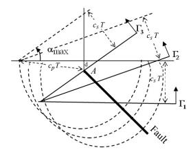
**Figure 3.** Adjoint S-waves propagating upwards. The angles between the propagating vectors and the vertical depend on the depth d of the nearest point A to the ground. The maximum angle is for the front  $\Gamma_3$ , the minimum (zero value) for the front  $\Gamma_1$ .
