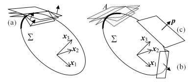
**Figure 4.** Left: adjoint S-waves propagating upwards (a) with different p under some angle constraints for determining the tangents to the fault front near point A. Right: P-waves of arbitrary propagation vectors (b) can also be used for determining the fault plane. A P-wave parallel to the fault plane (c) is used to determine the fault geometry.
