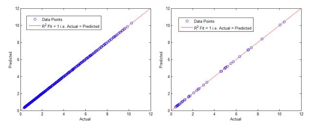
**Figure 6.** Simulated percentage change in natural frequencies:  $R^2$  plot between actual and the predicted output from the ANN model for mode-1 training (left) and testing (right) datasets.
