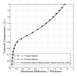
Figure 2. Deflection versus compression loads.
