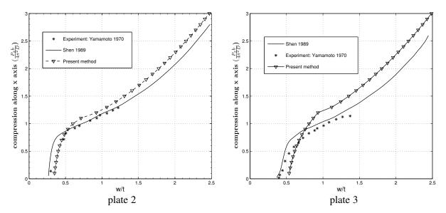
**Figure 9.** Uniaxial compression versus maximum deflection with a constant lateral pressure by the present method, the perturbation method [Shen 1989] and the experiment [Yamamoto et al. 1970]. Axial load versus deflection: plate 2 (left) and plate 3 (right).
