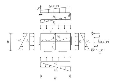
Figure 1. A rectangular plate with initial deflection and general in-plane and lateral loads.
