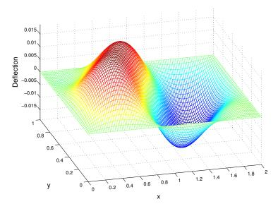
**Figure 12.** Deformation of a rectangular plate under uniaxial compression  $P_x = 0.65 P_{\text{xcr}}$  (applied first and keep constant) and shear  $\tau = 2\tau_{\text{cr}}$  (applied gradually).
