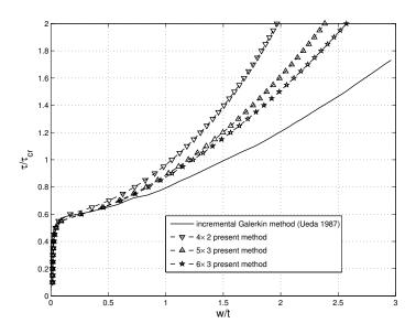
**Figure 14.** Comparisons of load-deflection curves as given by present global Galerkin method and the incremental Galerkin method [Ueda et al. 1987] under uniaxial compression combined with a shearing load.
