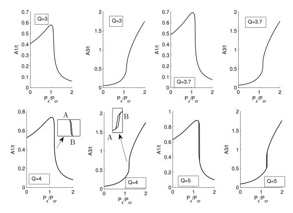
Figure 10. The deflection versus axial load relationships for a range of lateral loading Qs: Q = 3, 3.7, no hysteresis; Q = 4, 5, hysteresis occurs.
