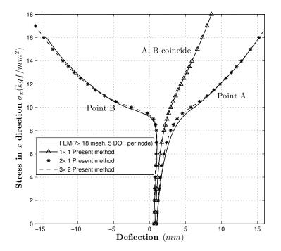
**Figure 4.** Stress  $\sigma_x$  versus deflection of point A and B, for the present Galerkin method and the finite element method.
